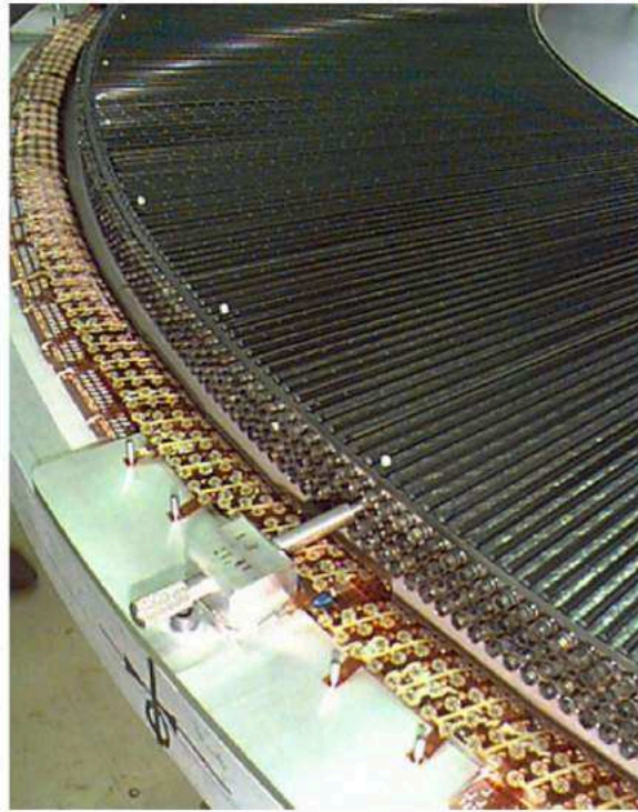
Fig. 3.9: Photograph of TRT endcap wheel during assembly. The inner and outer C-fiber rings can be seen, as well as the first layer of straws and the first stack of polypropylene radiator foils beneath it [8].
