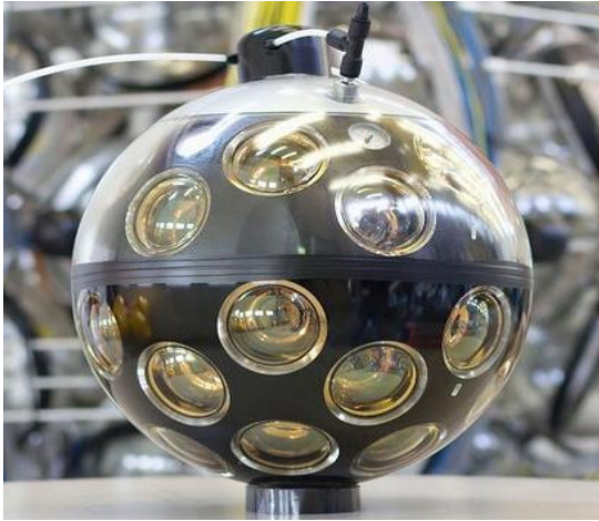
Figure 2.7: A photograph of a completed DOM.
