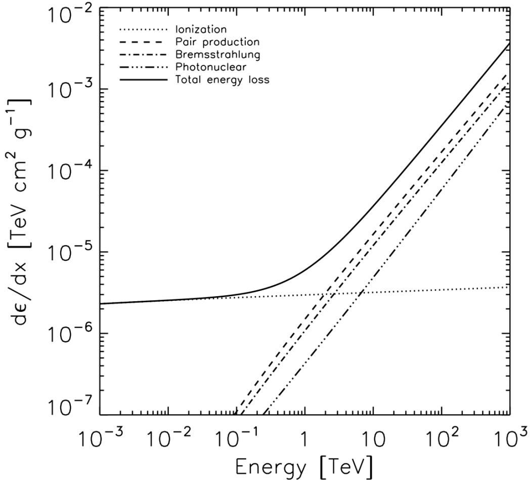
**Figure 5.6:** Theoretical predictions of the different contributions to the energy loss of high energy muons in water. The total energy loss (solid line) is decomposed into contributions from different processes, indicated in the legend [132].
