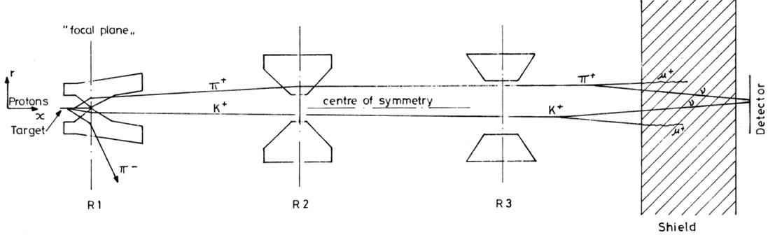
**Figure 1.7:** Schematic representation of an accelerator neutrino experiment [24].
