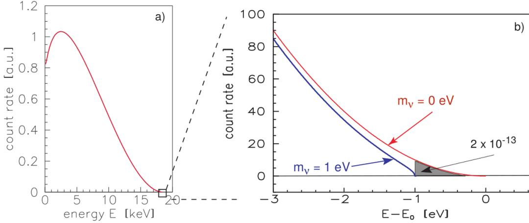
**Figure 1.22:** The electron energy spectrum of Tritium  $\beta$ -decay: complete (a) and narrow region around the endpoint  $E_0$  (b). The  $\beta$  spectrum is shown for neutrino masses of 0 and 1 eV [94].
