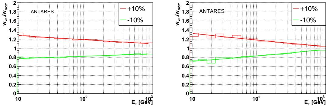
**Figure 6.5:** Expected event weight corrections as a function of true neutrino energy for a +10% (red) and -10% (green) from the nominal value of the OM photon detection efficiency. Left panel:  $\nu_\mu + \bar{\nu}_\mu$  CC events; Left panel:  $\nu_e + \bar{\nu}_e$  CC events.
