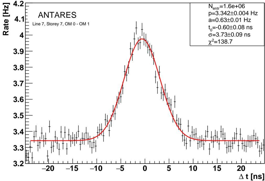
**Figure 3.1:** Example of the detected hit time differences,  $\Delta t$ , between two adjacent OMs. The fitted parameters are listed as well (see Equation 3.5 for details). The plot refers to one pair of OMs in the same storey (Line 7, Storey 7, OM 0 - OM 1) for one of the periods considered in the analysis.
