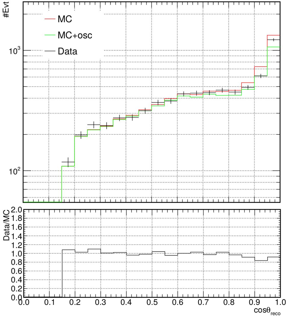
**Figure 6.10:** Data/MC comparison for reconstructed cosine of zenith. MC events have been weighted both assuming no oscillations (red), and assuming a simple 2-flavour oscillation scenario, with  $\Delta m_{32}^2 = 2.46 \times 10^{-3} \text{ eV}^2$  and  $\theta_{23} = 41.38^\circ$  (green). The Data/MC ratio is computed using MC without oscillations.
