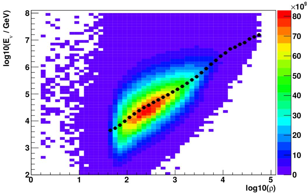
**Figure 5.7:** The correlation between the reconstructed  $dE/dX$  and the true energy is used to calibrate the energy estimator. The black markers denotes the derived calibration table, i.e. the average true energy per  $dE/dX$  bin [133].
