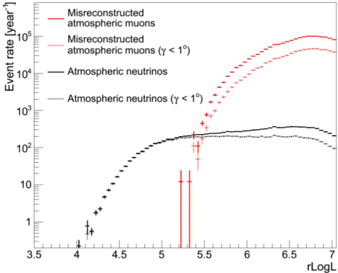
**Figure 5.4:** Distributions of the  $r \log L$  variable of *GridFit* for events reconstructed as up-going: atmospheric neutrinos (black) and misreconstructed atmospheric muons (red). An additional cut in  $\beta_{Grid}$  ( $\gamma$  in the figure) has also been applied (softer points) [130].
