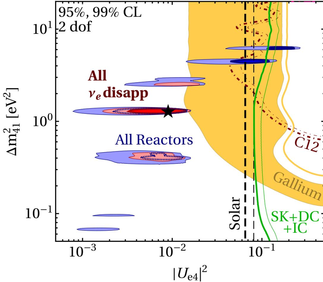
**Figure 1.12:** Constraints on  $\nu_e/\bar{\nu}_e$  disappearance in the 3+1 scenario. The preferred parameter regions at 95% and 99% CL are shown, projected onto the plane spanned by the mixing matrix element  $|U_{e4}|^2$  and the mass squared difference  $\Delta m_{41}^2$ . The parameter space inside the shaded areas and to the left of the exclusion curves is allowed. For details on the included data and the followed procedure, see [65].
