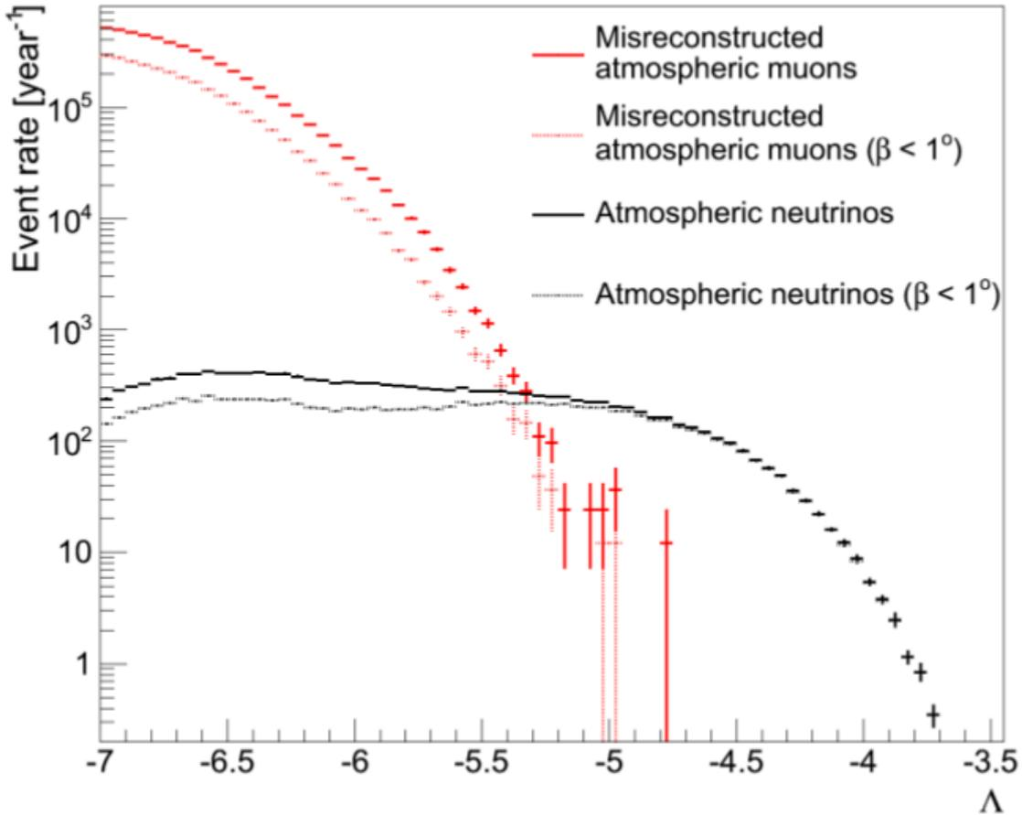
**Figure 5.2:** Distributions of the  $\Lambda$  variable of *AAFit* for events reconstructed as up-going: atmospheric neutrinos (black) and misreconstructed atmospheric muons (red). An additional cut in  $\beta_{AA}$  has also been applied (softer points) [130].
