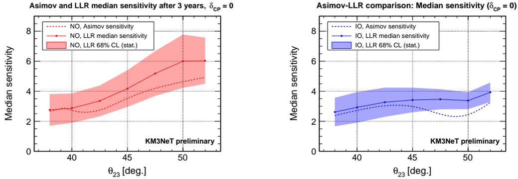
**Figure 1.19:** Expected median sensitivity of the KM3NeT/ORCA detector after 3 years of data taking in discarding the wrong mass ordering, as a function of the true value of  $\theta_{23}$ . Two different methods have been tested, namely an Asimov test approach and a log-likelihood ratio (LLR) [77].
