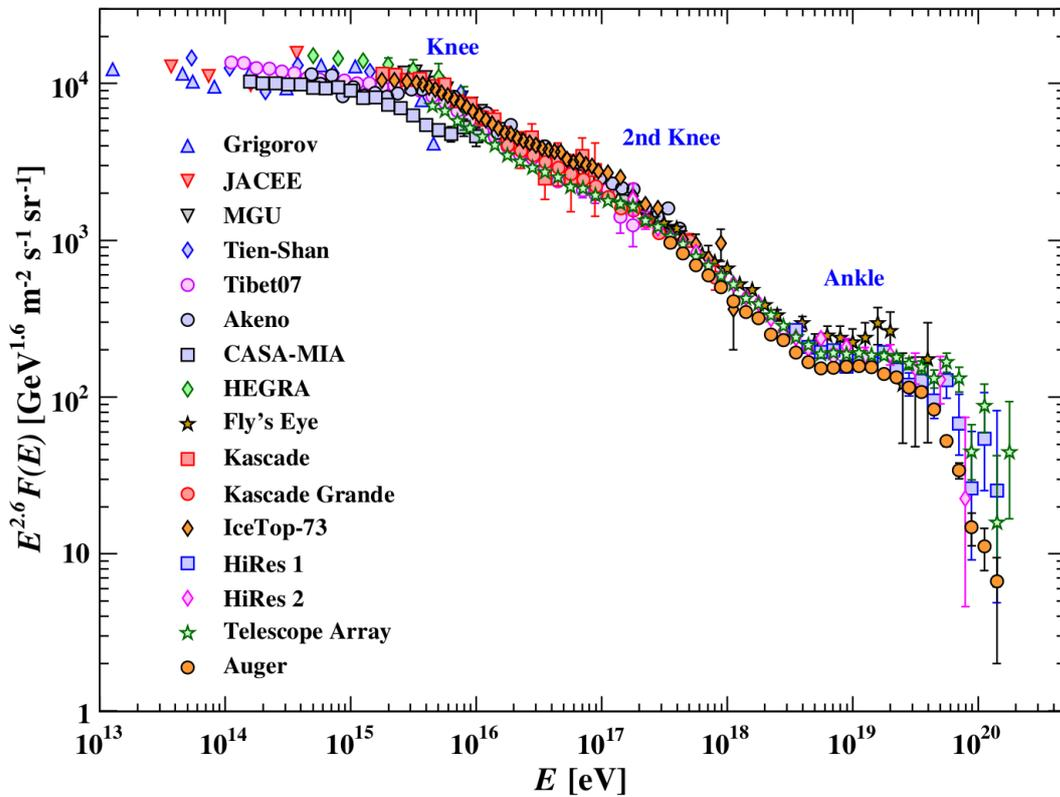
**Figure 1.5:** The all-particle spectrum as a function of  $E$  (energy-per-nucleus) from air shower measurements. The differential energy spectrum has been multiplied by  $E^{2.6}$  in order to display the features of the steep spectrum that are otherwise difficult to discern [15].
