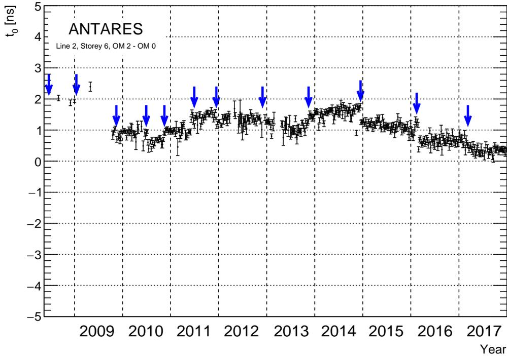
**Figure 3.5:** Fitted time offset as a function of time for one OM pair (Line 2, Storey 6, OM 2 - OM 0). The blue arrows indicate the periods in which high voltage tuning of the PMTs has been performed.
