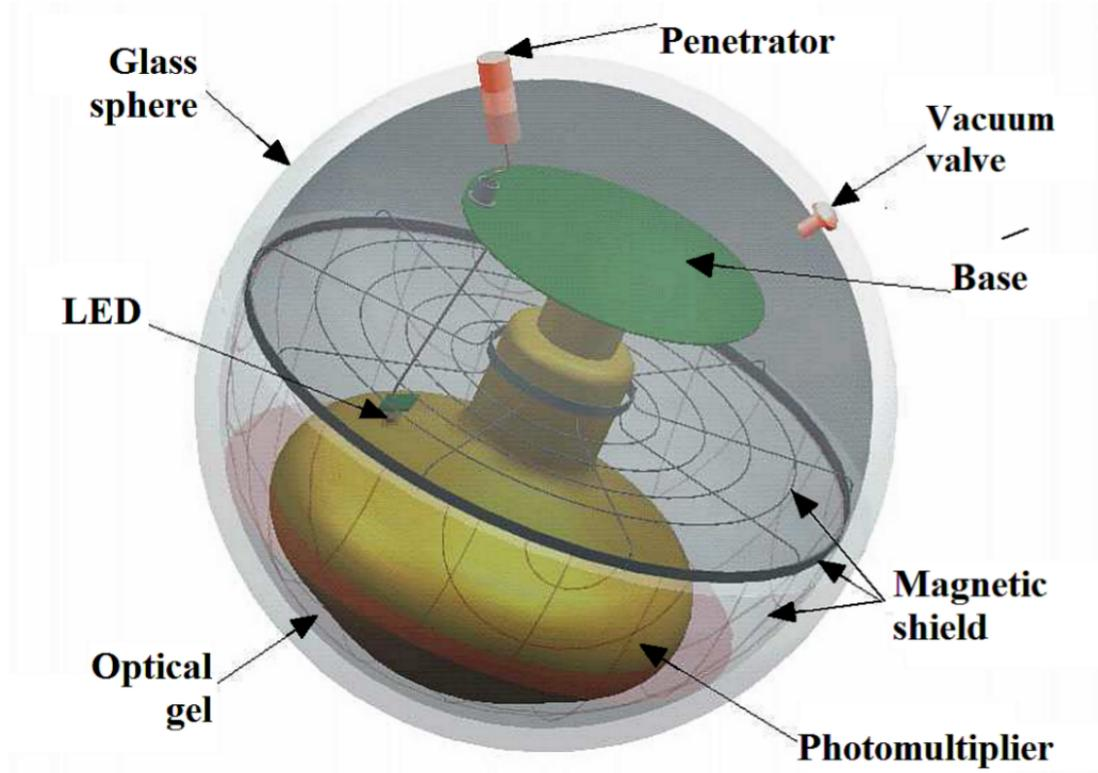
Figure 2.3: Schematic representation of an ANTARES OM [99].
