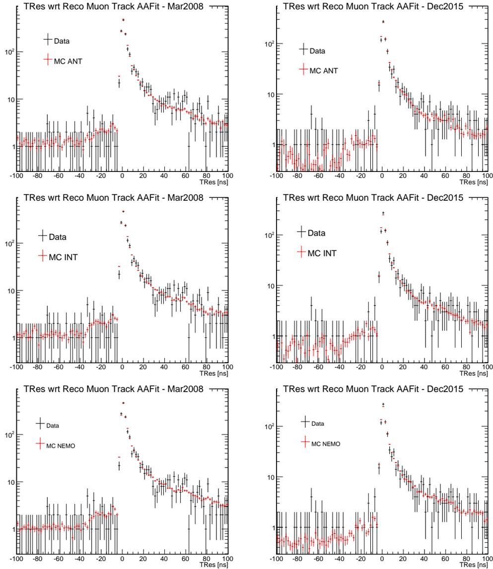
**Figure 4.4:** From top to bottom: *antares*, *intermediate* and *nemo* MC productions vs data; from left to right: the two analyzed periods, March 2008 and December 2015. Histograms are in 100 bins of 2 ns, and MC are normalized with the ratio between the number of entries of data and MC itself.
