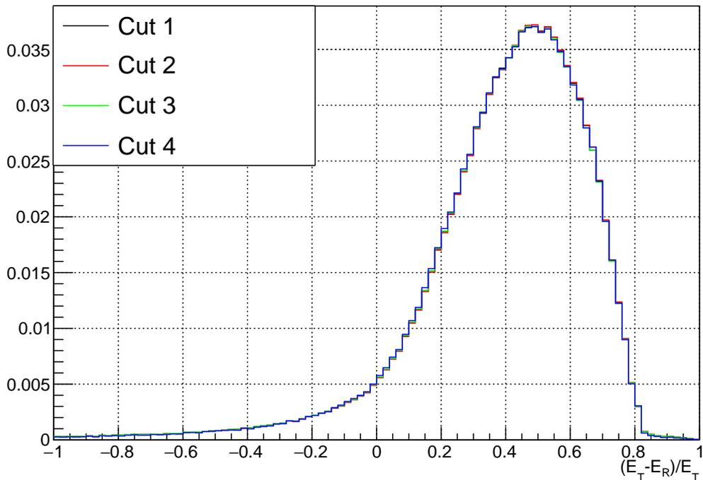
**Figure 5.8:** Energy resolution for MC  $\nu_\mu$  and  $\bar{\nu}_\mu$  CC events with true energy below 100 GeV.  $E_T$  is the true neutrino energy, while  $E_R$  is the reconstructed one. Different colors stand for different sets of event selection criteria. The distributions have been normalized to one.
