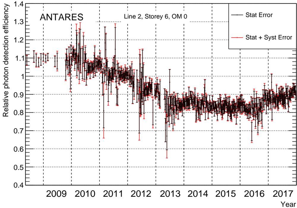
**Figure 3.2:** Photon detection efficiency as a function of time for one ANTARES OM (Line 2, Storey 6, OM 0). Error bars correspond to statistical (black) and statistical plus systematic (red) contributions.
