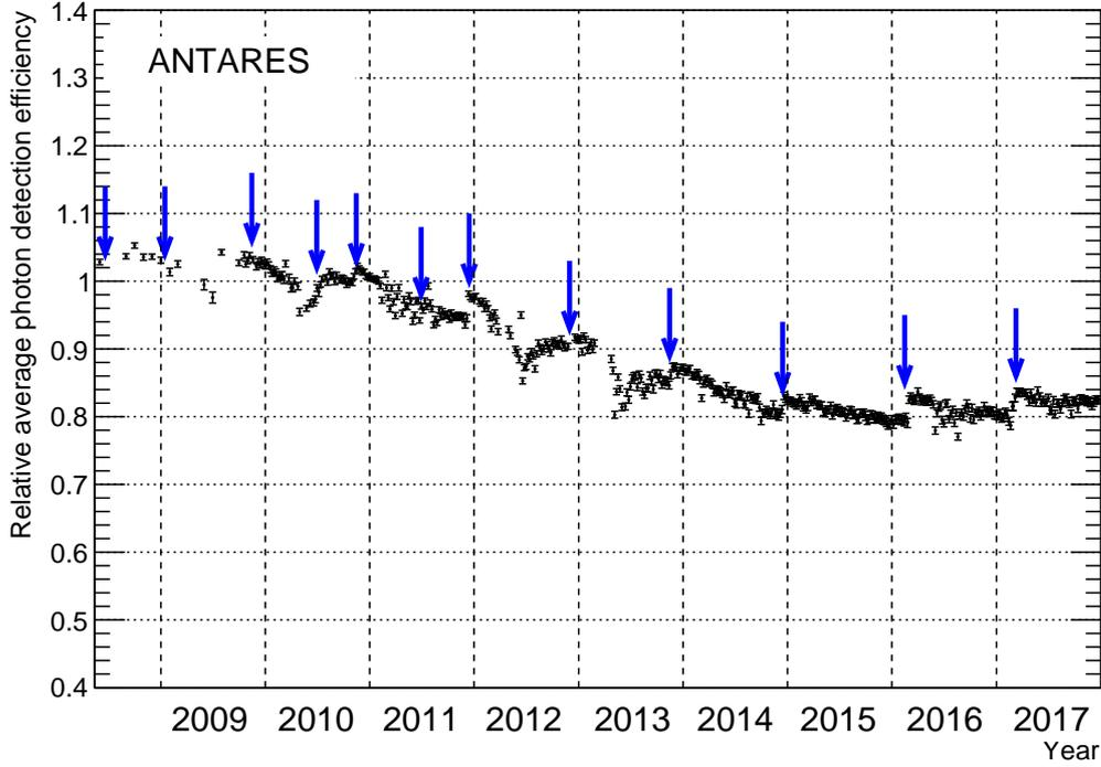
**Figure 3.3:** Relative OM efficiency averaged over the whole detector as a function of time. The blue arrows indicate the periods in which high voltage tuning of the PMTs has been performed, while error bars indicate the statistical error  $\sigma_{\text{mean}}$  on the mean efficiency.
