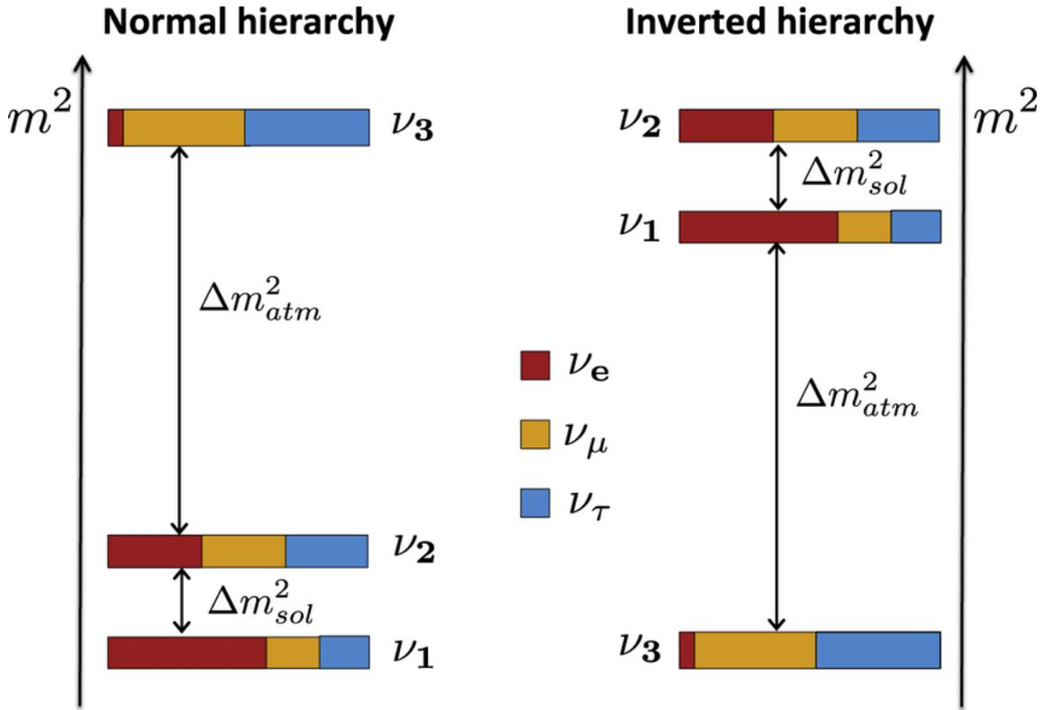
**Figure 1.18:** Scheme of the two distinct neutrino mass hierarchies. The colour code indicates the fraction of each flavour ( $e$ ,  $\mu$ ,  $\tau$ ) present in each of the mass eigenstates ( $\nu_1$ ,  $\nu_2$ ,  $\nu_3$ ) [53].
