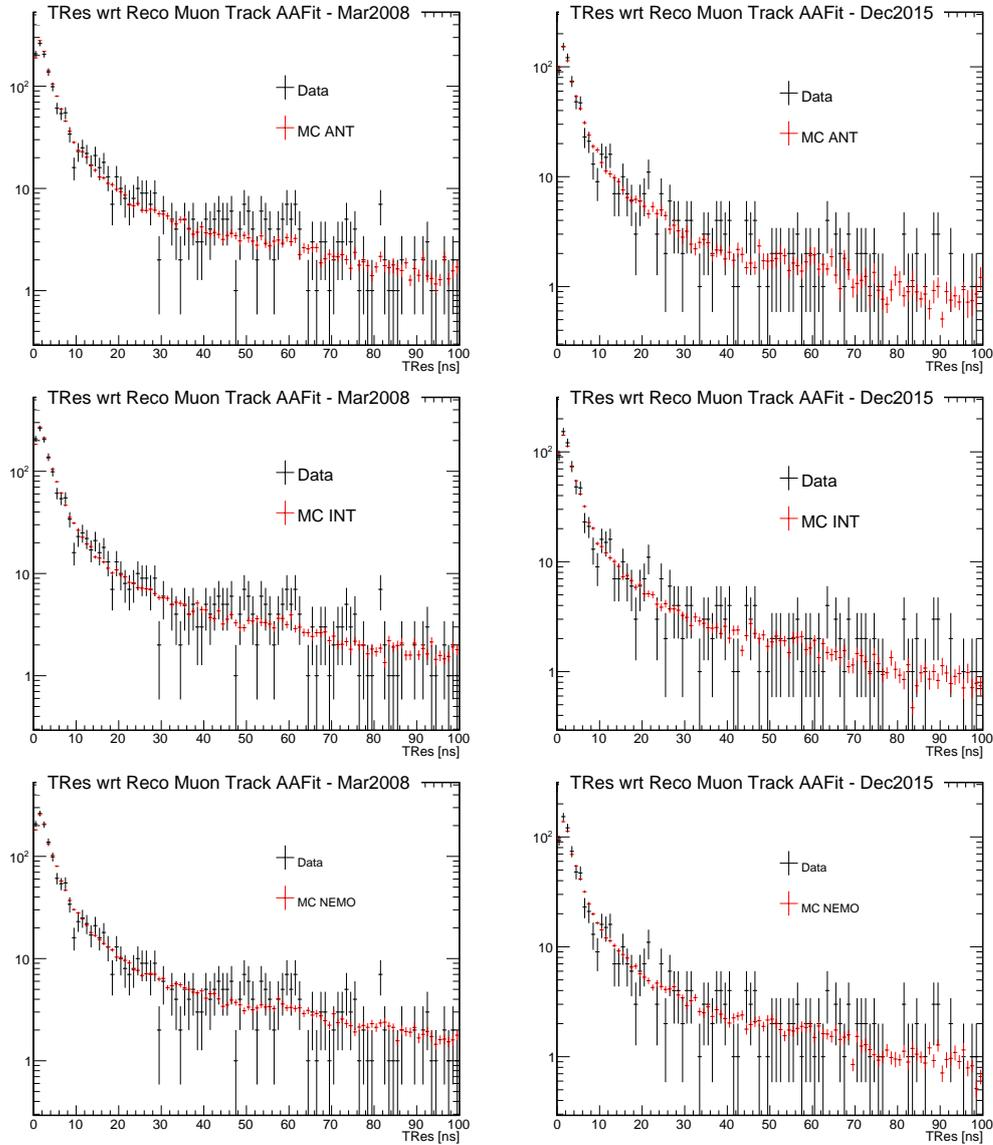
**Figure 4.3:** From top to bottom: *antares*, *intermediate* and *nemo* MC productions vs data; from left to right: the two analyzed periods, March 2008 and December 2015. Histograms are in 100 bins of 1 ns, and MC are normalized with the ratio between the number of entries of data and MC itself.
