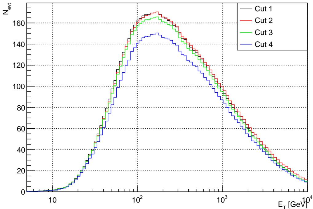
**Figure 5.9:** True energy distribution for MC  $\nu_\mu$  and  $\bar{\nu}_\mu$  CC events. Different colors stand for different sets of event selection criteria. The total number of expected events over the whole lifetime of data considered is also shown.
