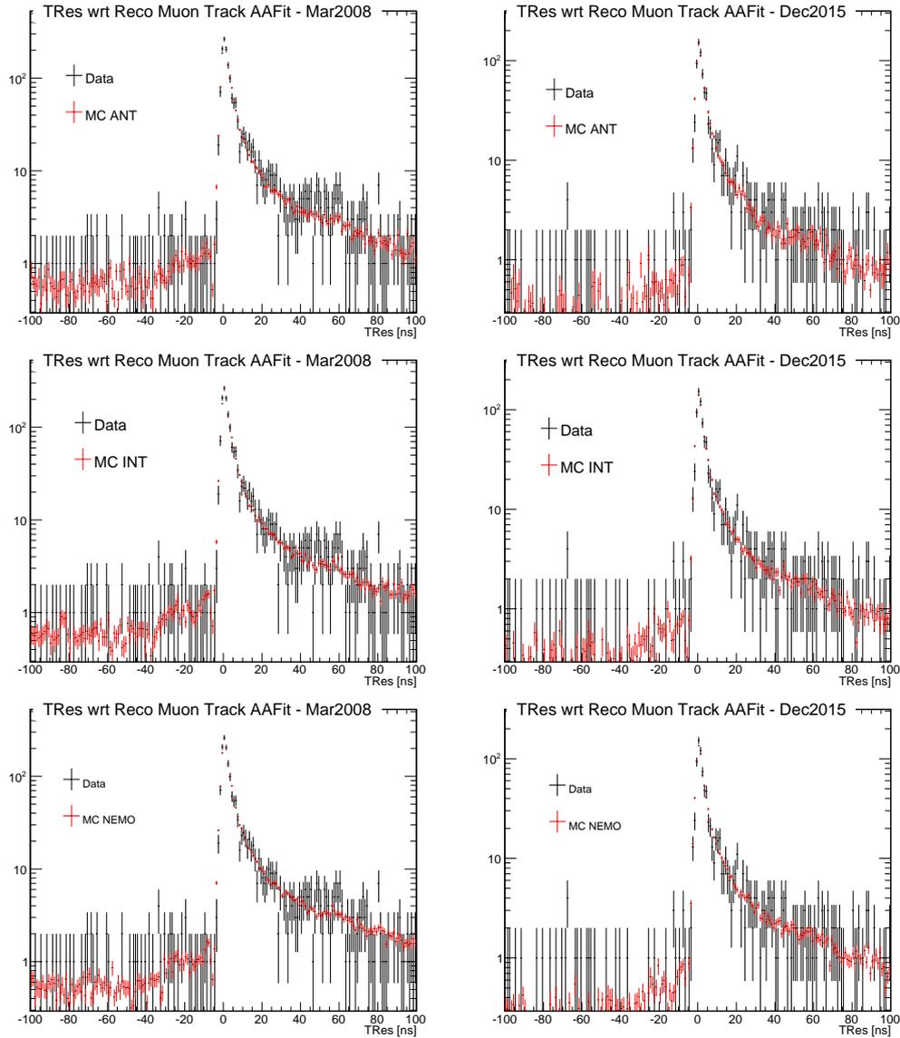
**Figure 4.2:** From top to bottom: *antares*, *intermediate* and *nemo* MC productions vs data; from left to right: the two analyzed periods, March 2008 and December 2015. Histograms are in 200 bins of 1 ns, and MC are normalized with the ratio between the number of entries of data and MC itself.
