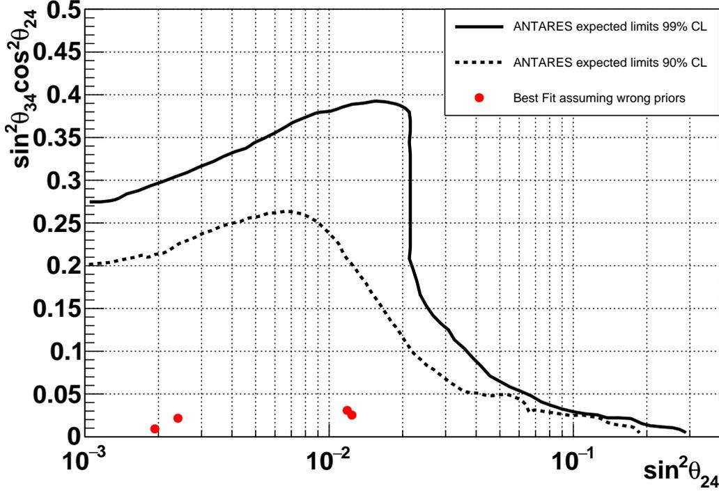
**Figure 7.1:** Expected 99% CL (solid line) and 90% CL (dashed line) exclusion regions for the 3+1 model parameters  $|U_{\mu 4}|^2 = \sin^2 \theta_{24}$  and  $|U_{\tau 4}|^2 = \sin^2 \theta_{34} \cos^2 \theta_{24}$ . Red dots are the global minima found for each of the performed tests with "wrong" priors on  $\Delta m_{32}^2$  and  $\sin^2(2\theta_{23})$ . Exclusion regions are on the right-hand side of the curves.
