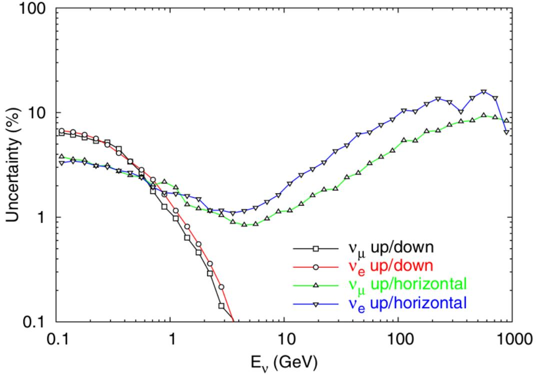
**Figure 6.3:** Uncertainties in directional ratios as a function of neutrino energy.  $\nu_{\mu,up}/\nu_{\mu,down}$  is shown with black lines with squares,  $\nu_{e,up}/\nu_{e,down}$  with red lines with circles,  $\nu_{\mu,up}/\nu_{\mu,hor}$  with green lines with triangles and  $\nu_{e,up}/\nu_{e,hor}$  with blue lines with triangles [14].
