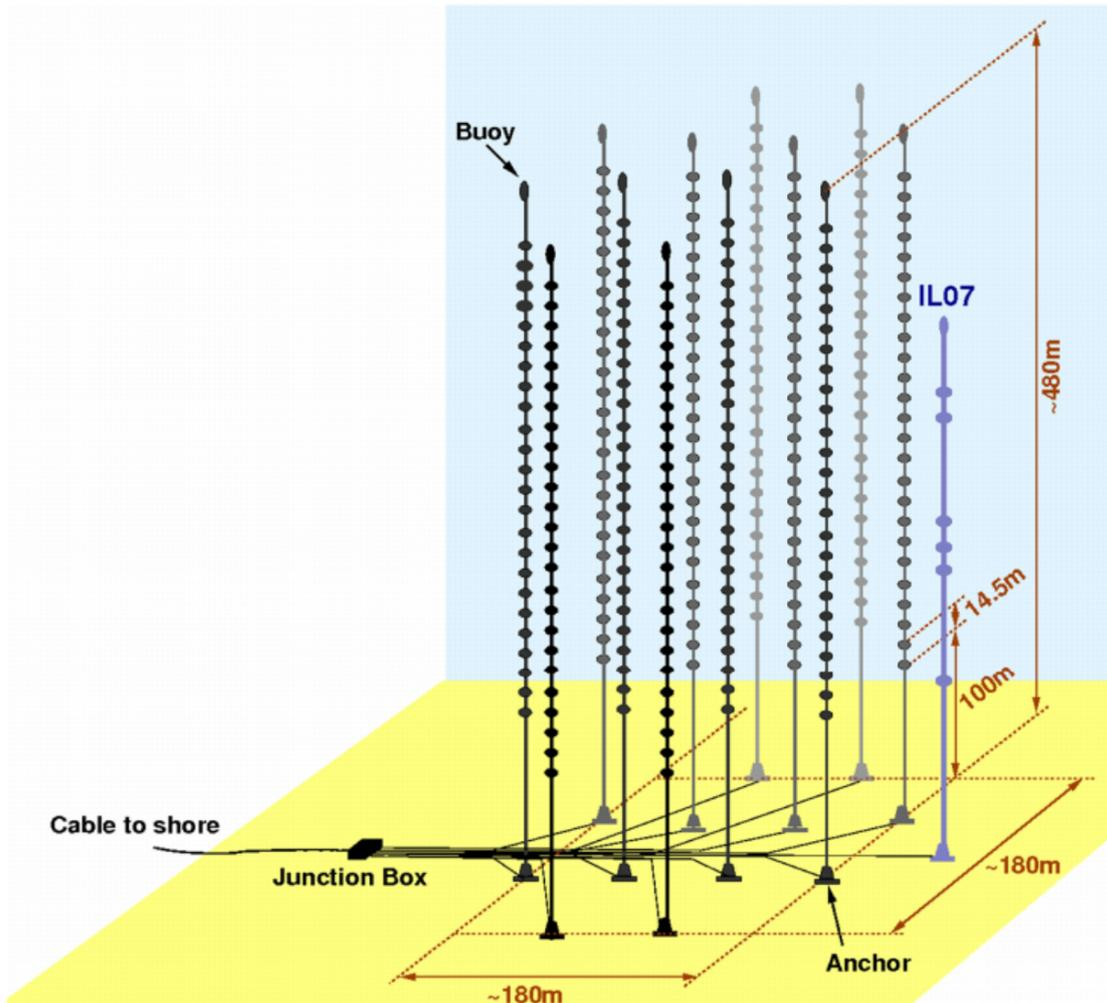
Figure 2.2: Schematic representation of the ANTARES layout [99].
