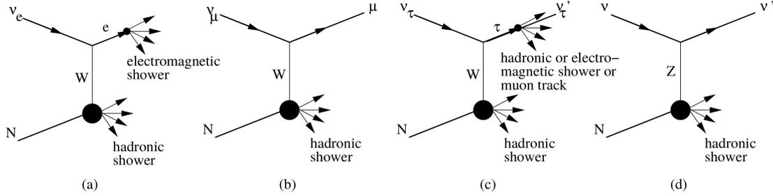
**Figure 1.9:** Neutrino-nucleon deep inelastic interaction channels. Charged current interactions of all three neutrino flavours (a-c) and neutral current interactions (d) identical for all neutrino flavours [27].
