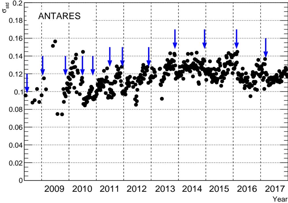
**Figure 3.4:** Standard deviation  $\sigma_{\text{std}}$  of the relative photon detection efficiency as a function of time. The blue arrows indicate the periods in which high voltage tuning of the PMTs has been performed.
