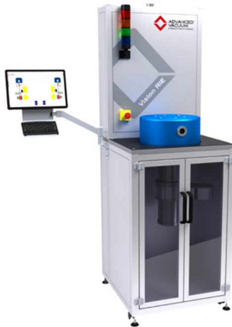
Figure 6.25: The "Advanced Vacuum-Vision 320" RIE machine used in this study to etch the TLM samples.
