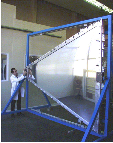
Figure 36: One MDC-IV in construction at IPN Orsay
