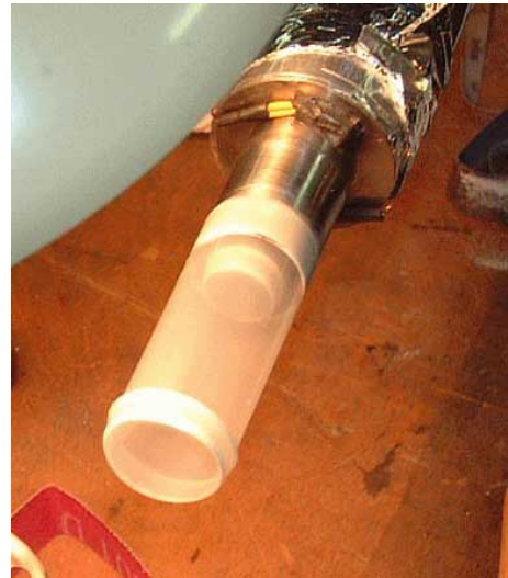
Figure 34: Picture of the Liquid-hydrogen target vessel. The entrance window is glued on a stainless-steel tube.
