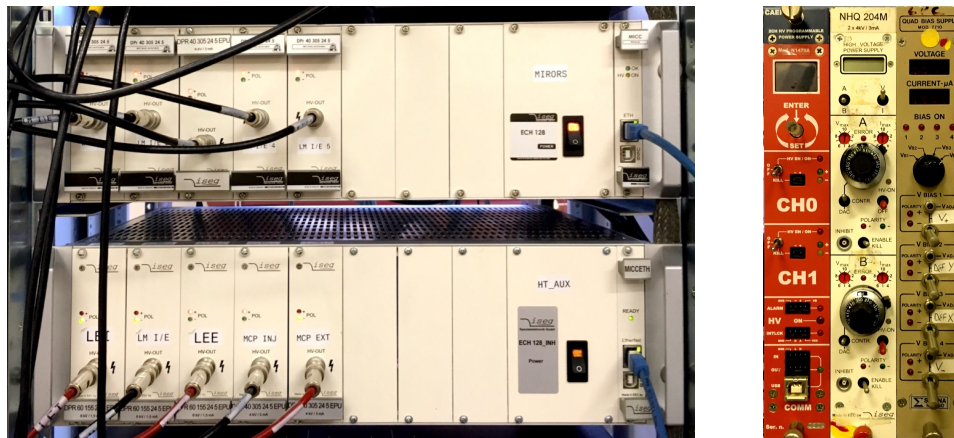
Figure 4.3 – Control and monitoring user interface for the high voltage power supplies and the pulse generation.
