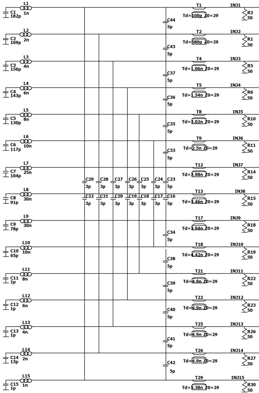
Figure 28: Typical simulation schematic when injecting on channel 8. Crosstalk capacitances have only been set for channels in connection with channel 8.
