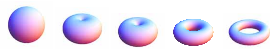
Figure 8. Pumpkin-like configuration versus the ratio s of the semi-axes and torus defined by the sausage r_s and torus r_t radii. The axis of revolution is the vertical axis.
