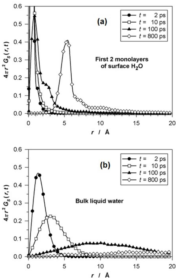
**Figure 5.** (a) Van Hove self-correlation functions for the diffusing H<sub>2</sub>O molecules in the first two monolayers of water at the surface of tobermorite. The VHSCF corresponding to the isotropic diffusion of H<sub>2</sub>O molecules in bulk liquid water is shown in (b) for comparison.
