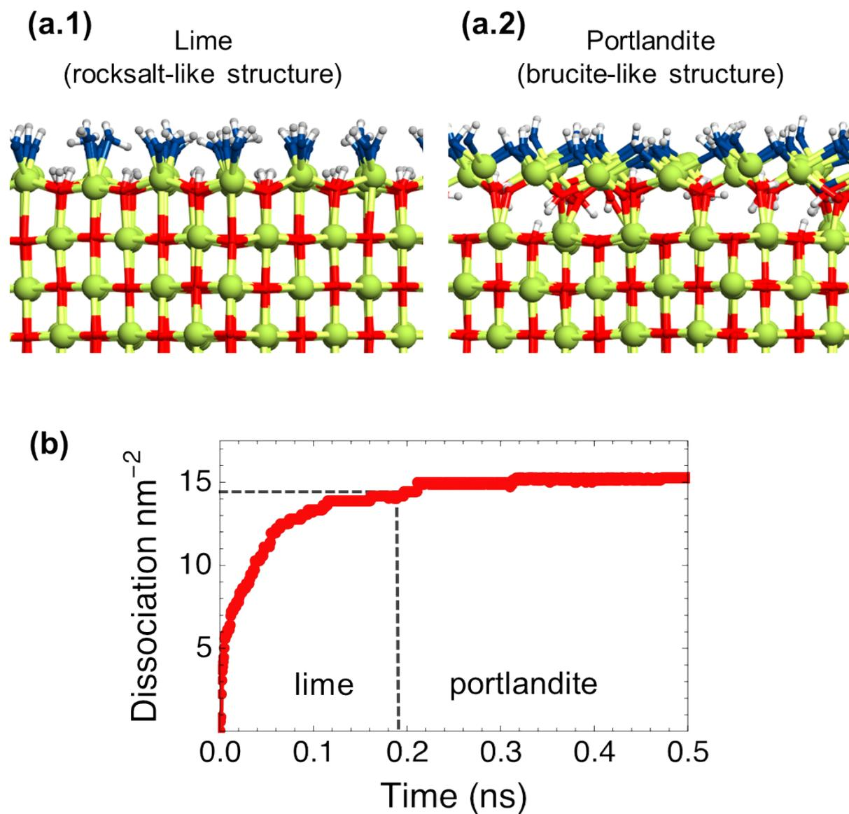
**Figure 9.** (a) Snapshots of the simulation. Ca is represented as green spheres, H as white spheres, and oxygen atoms from the solid and from water as red and blue spheres respectively. (a.1) Shows the structure at 0.15 ns, when water has reacted with the surface but the lime structure is maintained. (a.2) shows the structure at 0.25 ns, when the top layer has transform into portlandite. (b) Amount of water dissociated per  $\text{nm}^2$  as a function of time.
