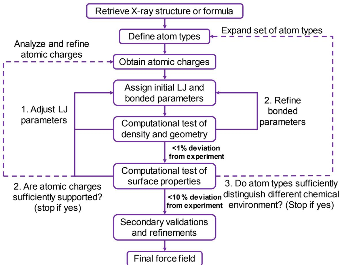
**Figure 2.** Procedure for parameterization of new compounds in the IFF, including the most common refinement loops. Careful assignments in every step of algorithm in full agreement with physical and chemical understanding minimize the need for loops. In principle, it is possible to go back to any prior step at each stage in the procedure until thermodynamic consistency is achieved. Adapted from [ref 44].
