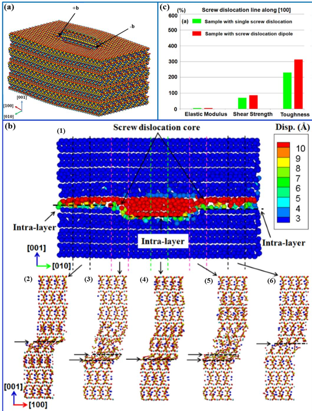
**Figure 12.** (a) Atomic configurations of the super cell of tobermorite samples containing screw dislocation dipole with opposite signs,  $+b$  and  $-b$ . The dislocation line is along  $[001]$ . (b) Atomic configurations of tobermorite with screw dislocation dipole along  $[100]$  at strain of
