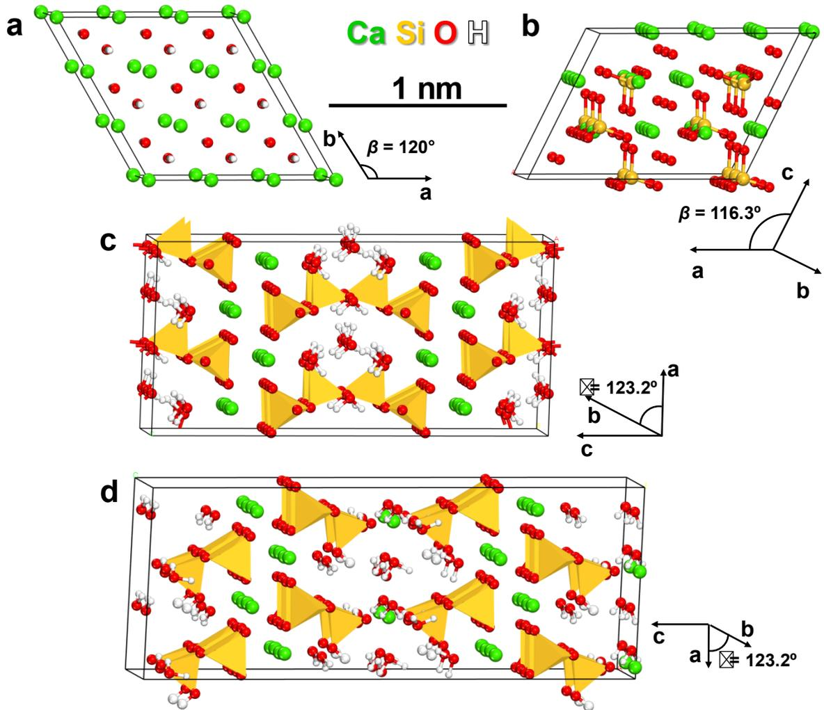
**Figure 3.** Crystal structures of selected cement minerals are shown. (a) portlandite (trigonal crystal system) [ref 142], (b)  $M_3$  polymorph of tricalcium silicate (monoclinic crystal) [ref 141], (c) tobermorite 11 Å [ref 143] and (d) tobermorite 14 Å (monoclinic crystal) [ref 131]. Lattice constants from XRD data are also presented in Table 1 for all minerals.
