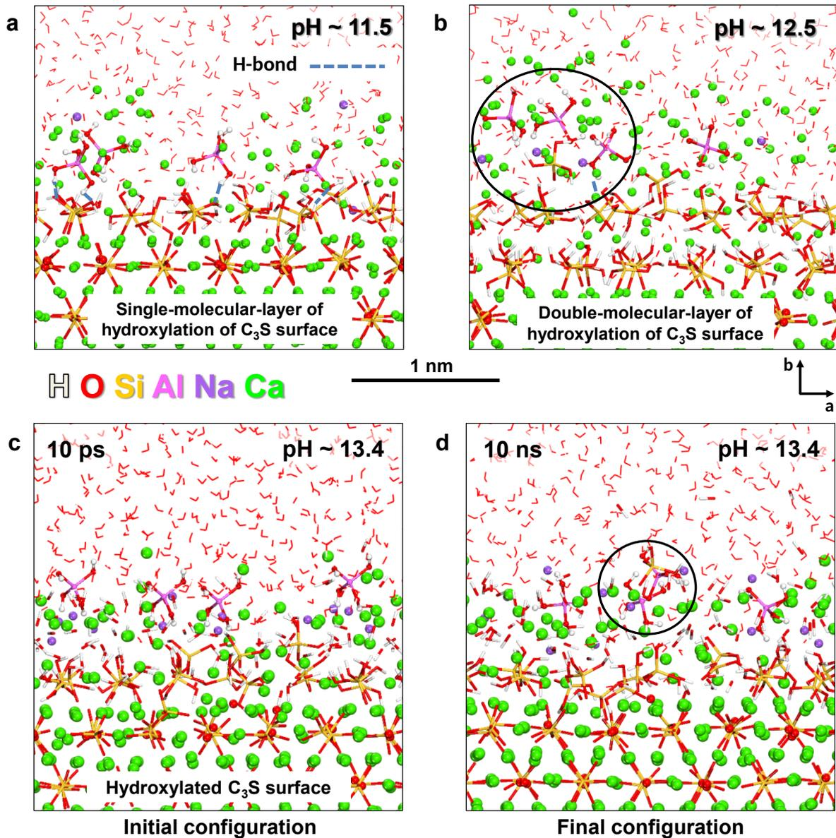
**Figure 7.** Interactions of aluminate ions with the hydroxylated C<sub>3</sub>S surface according to molecular dynamics simulation. (a) Interactions of aluminate ions with the initially hydrated C<sub>3</sub>S surface (one molecular layer) at pH ~ 11.5 involve strong bonding to calcium ions on the surface as well as interfacial hydrogen bonds (Al–OH···O<sup>-</sup>–Si and Al–OH···OH–Si). (b)
