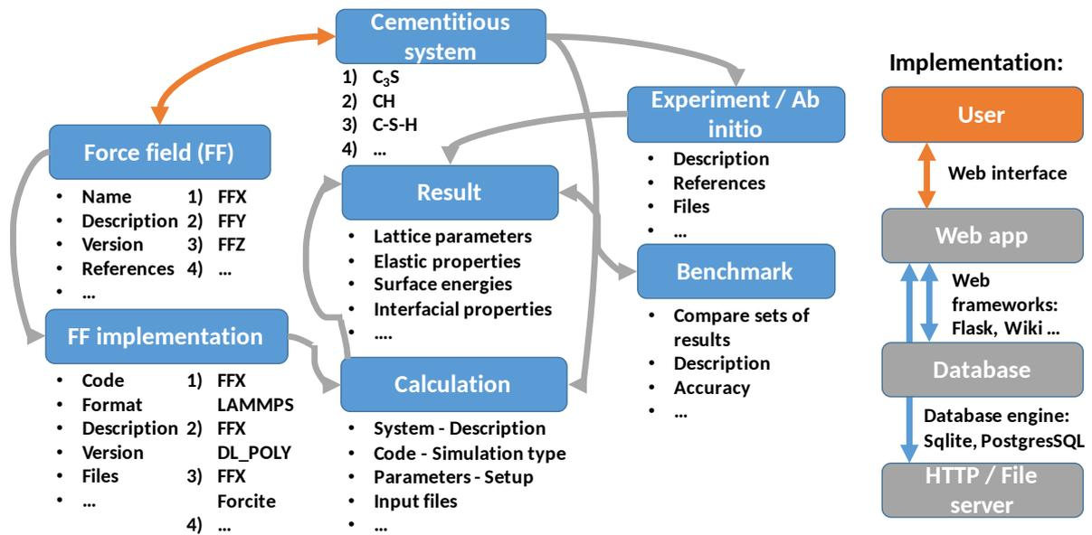
**Figure 1.** Schematic of CEMFF/*cemff* database structure which includes different types of force field models available for cementitious materials. Text boxes with blue color show the input and comparison sections.
