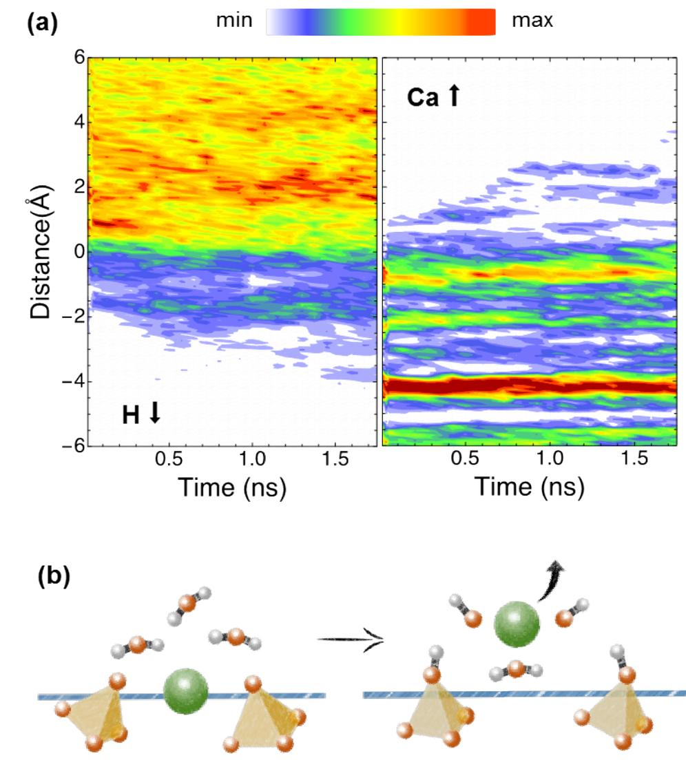
**Figure 11.** (a) Time resolved atomic density profiles of H and Ca on  $C_3S$  (010) surface. The distance origin shows the position of the Gibbs plane defining the position of the surface before hydration. Hence, negative values indicate positions inside the crystals. The color scale represents the element-normalized number of atoms at a given distance from the surface. (b) Schematic representation of the hydration process.
