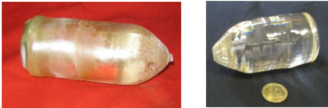
Fig. 1. CdWO 4 (mass 3 kg, left) and ZnWO 4 (≈1.3 kg, right) single crystals.
