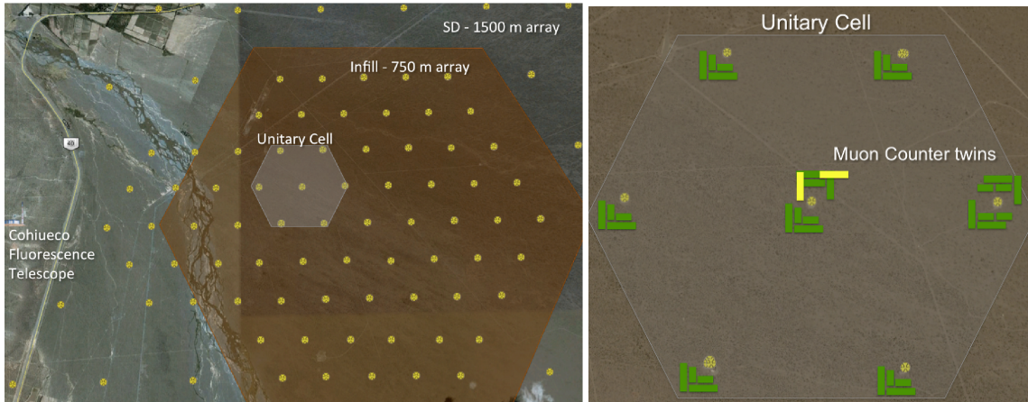
Figure 1. Left: Map of the AMIGA array with brown background (from [4]) with the Unitary Cell engineering array position (in gray). Right: layout of the Unitary Cell showing the locations of MCs and corresponding water-Cherenkov stations. Figure is not to scale. Green and yellow boxes represent MC modules buried at approximately 2.25 m and 1.3 m, respectively.
