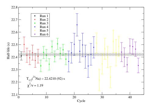
FIG. 3. (Color online) Half-life of <sup>21</sup>Na when data is analyzed on a cycle-by-cycle basis.
