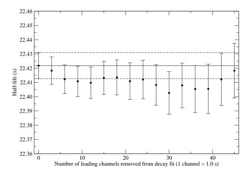
FIG. 2. Effect of removing an increasing number of leading channels on the <sup>21</sup>Na half-life (1 channel = 1.0 s) from the summed decay curve, with the half-life and uncertainty (22.4218 (92) s from Fig. 1) overlaid to guide the eye.
