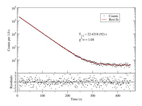
FIG. 1. (Color online) Decay curve of <sup>21</sup>Na and resulting global fit from the sum of all cycles and runs. The intensity of the fitted background is 41.6 (0.5) counts/s, representing a 0.97 (1) counts/s background rate in the scintillator. The fit residuals  $(y_i - y_{fit})/\sigma_i$  are displayed in the lower panel (mean of -0.0002 with a standard deviation of 1.02).
