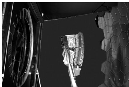
Figure 8: Photo of a fluorescence telescope at Coihueco.
