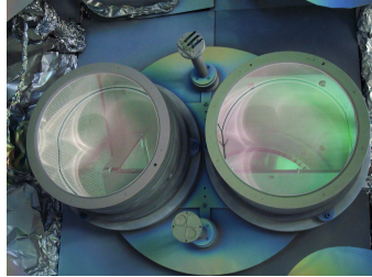
Figure 5. Planetary motion of the large substrates inside the coating chamber.
