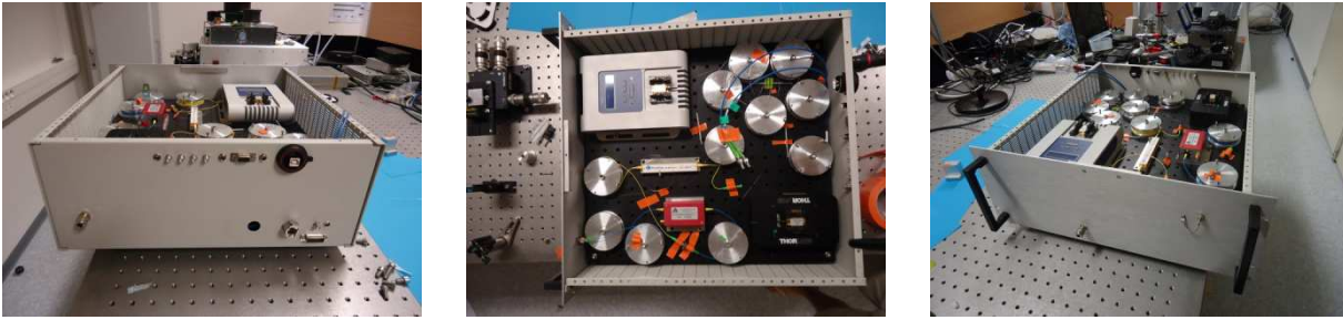
Figure 6.37. Pictures of the 52 W all-fibered setup integrated in a 19'' rack.
