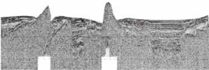
Figure 1. Typical seismic section (vertical scale: two-way travel time 0-4.5s, horizontal scale: distance) showing a rift with opposite tilted blocks.
