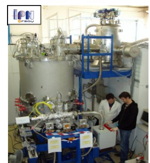
Figure 3: The SPIRAL2 superconducting cryomodules (left: \beta_0=0.07 – 1 cavity, right: \beta_0=0.12 – 2 cavities).
