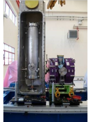
Figure 10: left - Laminar air flow in-between cryomodules in the linac tunnel, right – test of the assembly between a warm section and a CMA in Saclay.
