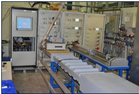
Figure 8: First cabinets of solid state amplifiers being tested at GANIL on the variable VSWR test bench.
