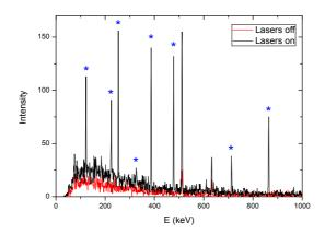
Figure 4: Typical  $\gamma$  spectra obtained at the tape station when the mass separator was set to select a mass-to-charge ratio A/Q= 106 with lasers on resonance for the ionization of tin (dark) and with lasers off (light). The asterisks indicate characteristic  $\gamma$  peaks from the  $\beta$  decay of  $^{106}$ Sn.
