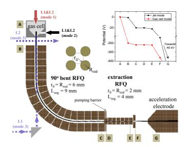
Figure 7: Schematic layout of the prototype RFQ ion-gude system tested at LISOL. Ion trajectories through the system obtained with the SIMION® software and the dimension of the RF electrodes are shown. The inset shows the evolution of the axial DC potential with reference to the different points indicated in the figure. Two alternative optical paths for laser ionization and spectroscopy are indicated (see text for details).
