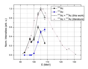
Figure 6: Normalized production intensities of <sup>212</sup>Ac and <sup>213</sup>Ac as a function of the energy of the primary beam at the exit of the target. The summed function of the two isotopes is also shown for comparison with previous experimental results (see text).
