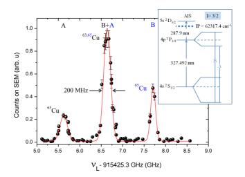
Figure 9: Hyperfine splitting of the  ${}^{2}P_{1/2}$  excited state for a natural abundance admixture of copper isotopes produced in the reference cell. The obtained linewidths were used to measure the reduction of the laser bandwidth by seeding of a CW diode laser into a pulse dye amplifier. The inset shows the ionization scheme employed in these tests and the expected HFS of the electronic levels.
