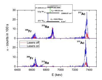
Figure 5: Alpha spectra obtained when the mass separator was set to select ions with A/Q= 212 (top) and 213 (bottom). Characteristic lines for  $^{212}$ Ac (E= 7380 keV) and  $^{213}$ Ac (E= 7364 keV) may be seen for lasers on (blue) and lasers off (red). The main contaminant species along with the daughter decay products are also observed. The ionization scheme used in the production of the Ac beams is shown on top.
