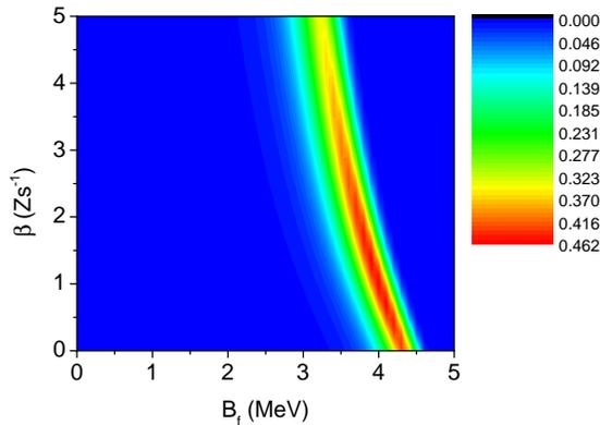
**Figure 3.** Probability density function of  $B_f$  and  $\beta$ . The true value of  $B_f = 4$  MeV and of  $\beta = 2 \times 10^{21} \text{ s}^{-1}$ . The number of data points is fixed to 3 and the experimental precision is 50%.
