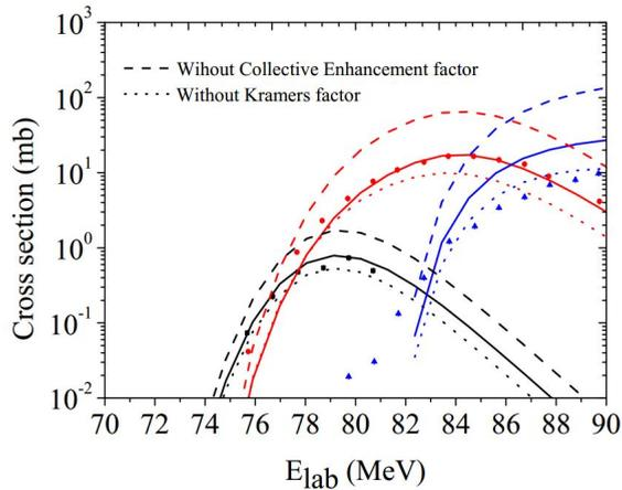
**Figure 2.** 2n, 3n and 4n fusion-evaporation cross-sections of the  $^{208}\text{Pb}(^{16}\text{O},xn)^{224-x}\text{Th}$  reaction as a function of energy. The solid curve corresponds to the reference model with Strutinsky-Kramers and collective enhancement factor. Dotted and dashed curves correspond to the same calculation without Kramers-Strutinsky factor or the collective enhancement factor, respectively. Data from Ref. [6] are also indicated.
