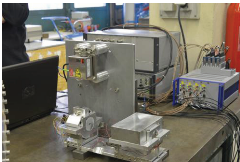
Figure 3: Calibration and stability studies of mechanical assembly with piezo-movers supporting the third IP-BPM.
