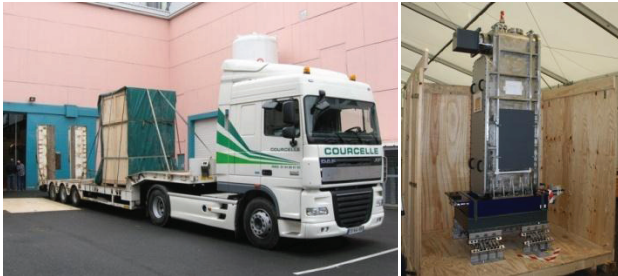
Figure 4: Transportation test of the cryomodule CMA2 from Saclay to GANIL. Right picture shows the cryomodule inside his crate, fixed on its damping support.
