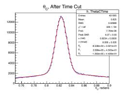
Figure 7: MC simulation of FDIRC expected Cherenkov angle resolution in CRT for H-8500 tube with 6 mm pixels and no chromatic correction.
