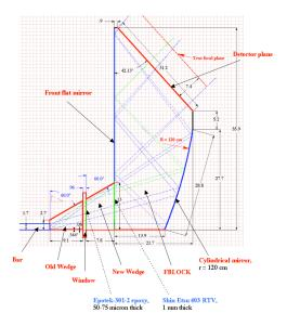
Figure 1: Optical design of FDIRC photon camera.
