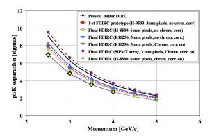
Figure 8: Final FDIRC expected PID performance for various detector options compared to the BaBar DIRC performance.
