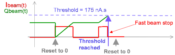
Figure 4: Principle of beam loss measurement integration.
