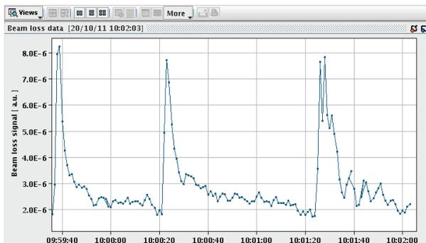
Figure 5: Closing the primary collimators to  $5\sigma$ . Loss rates recorded as a function of time for three  $10\mu\text{m}$  (or  $0.036\sigma$ ) steps, in 90 m operation at the 20 October 2011 at 10:02.
