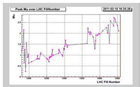
From the end of spring 2011, the number of bunches in the machine is high enough so that we are limited by the instantaneous luminosity the detectors can sustain, almost twice the nominal value. A levelling system has been developed together with the LHC operation team, so that our luminosity is kept constant by frequently adjusting the vertical separation of the beams. The nearby plot shows the exponential decay of the luminosity at ATLAS and CMS and our constant (lower) luminosity in red.
