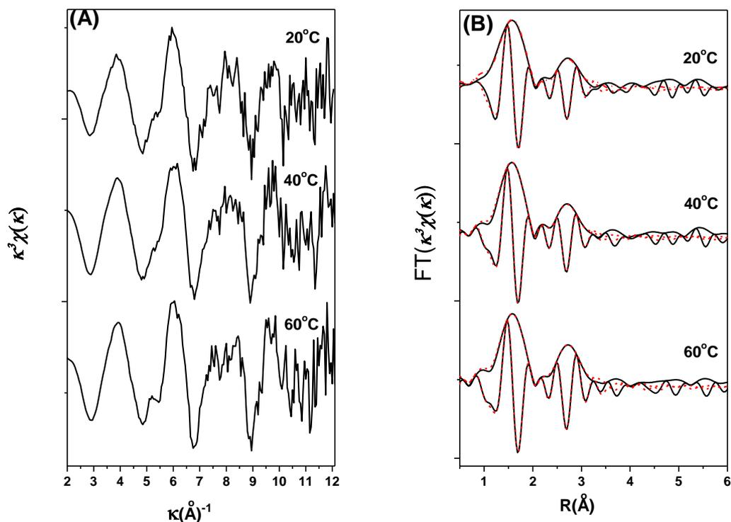
**Fig. SI-4** Raw  $k^3$ -weighted  $\chi(k)$  spectra of experimental samples (A) and their corresponding pseudo radial distribution functions (RDFs) (B) at three different temperatures.  $m/V = 0.5$  g/L,  $C_{\text{Ni(II)initial}} = 10$  mg/L,  $\text{pH} = 7.5$ ,  $T = 20, 40$  and  $60$  °C,  $I = 0.001$  mol/L.
