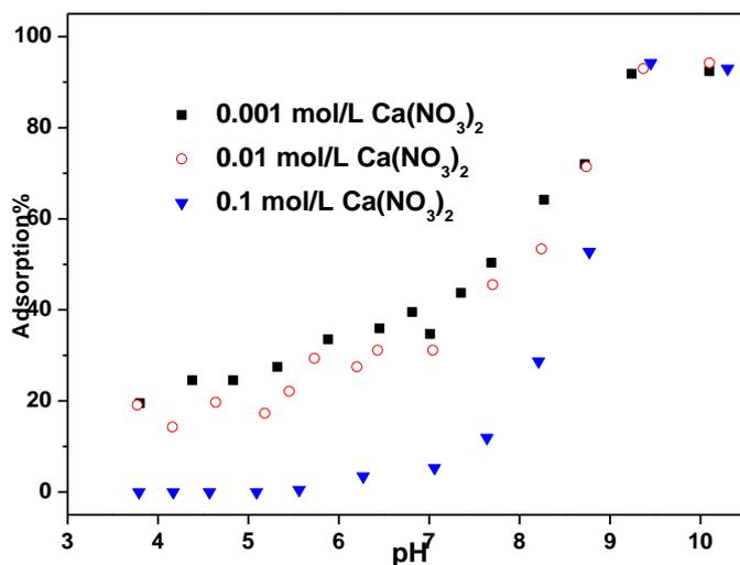
**Fig. SI-2** Sorption edges of Ni(II) at different ionic strengths.  $m/V = 0.5$  g/L,  $C_{\text{Ni(II)initial}} = 10$  mg/L,  $T = 20$  °C and  $I = 0.001, 0.01$  and  $0.1$  mol/L  $\text{Ca}(\text{NO}_3)_2$ .
