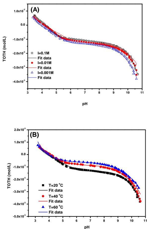
**Fig. SI-1** Acid-base titrations of Ca-montmorillonite (5.0 g/L) as a function of pH in 0.001, 0.01 and 0.1 mol/L  $\text{Ca}(\text{NO}_3)_2$  at  $T = 20\text{ }^\circ\text{C}$  (A) and at three different temperatures in 0.001 mol/L  $\text{Ca}(\text{NO}_3)_2$  (B). The lines are calculated using FITEQL 3.2.
