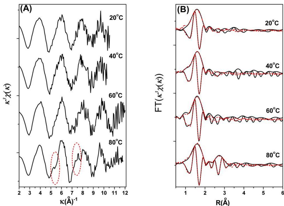
**Fig. 4** Raw  $k^3$ -weighted  $\chi(k)$  spectra of experimental samples (A) and their corresponding pseudo radial distribution functions (RDFs) (B) at three different temperatures.  $m/V=0.5 \text{ g/L}$ ,  $C_{\text{Ni(II)initial}}=10 \text{ mg/L}$ ,  $\text{pH}=6.4$ ,  $T=20, 40, 60$  and  $80^\circ\text{C}$ ,  $I=0.001 \text{ mol/L Ca(NO}_3)_2$ .
