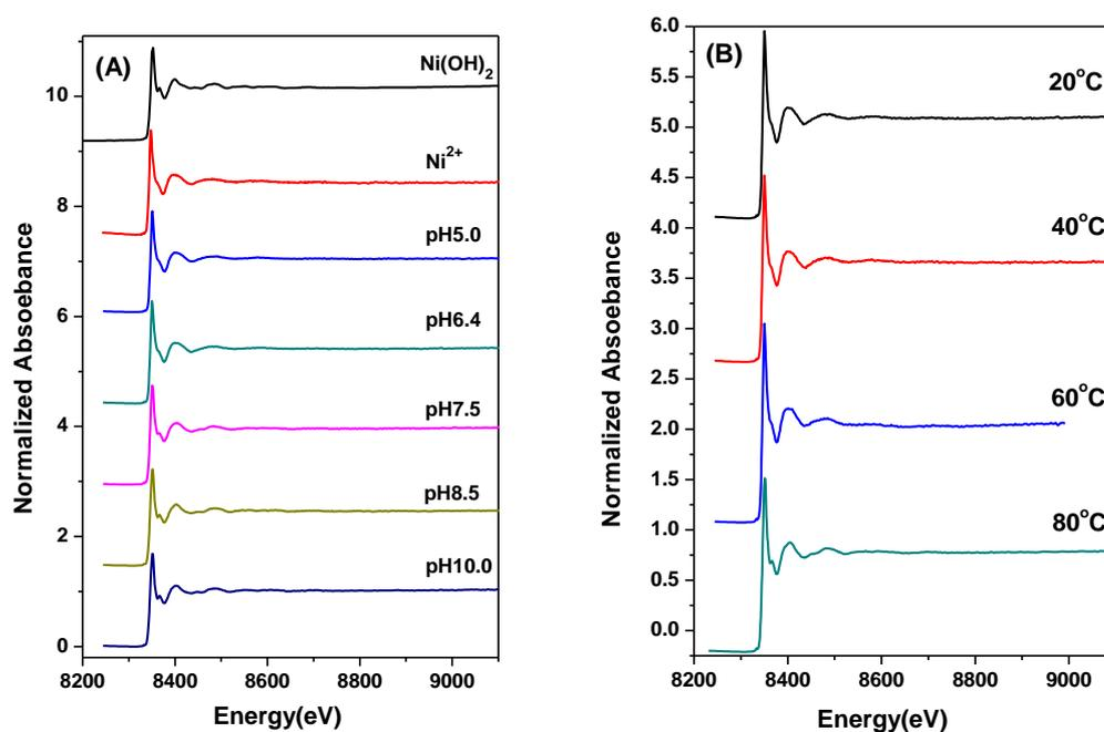
**Fig. SI-3** XANES spectra of the reference and sorption samples at different pH (A) and temperature (B).
