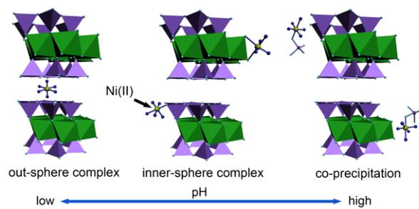
Sorption speciation of Ni(II) onto Ca-montmorillonite varies with pH.
