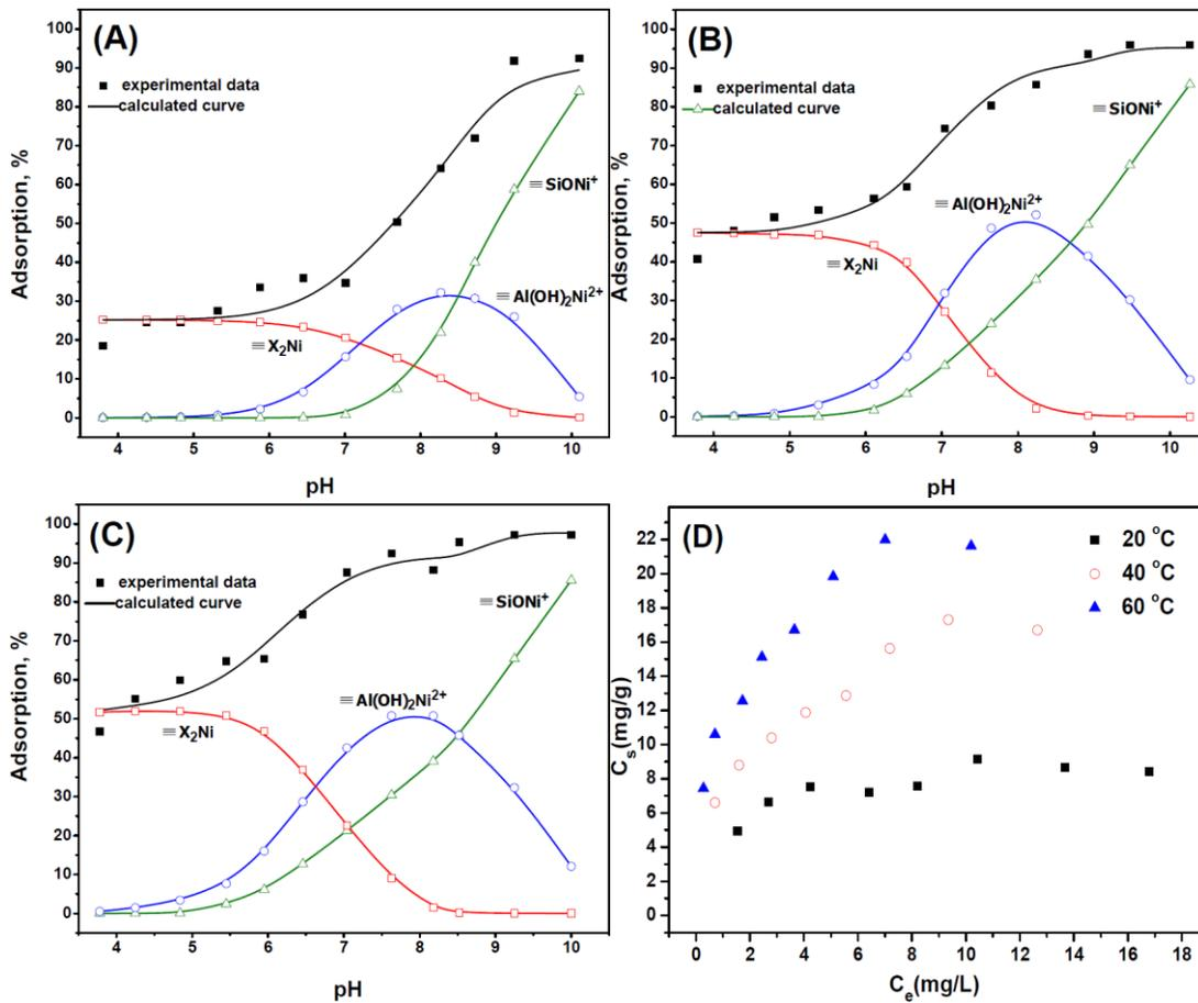
**Fig. 2** Sorption percent of Ni(II) on Ca-montmorillonite and corresponding surface species repartition diagrams at temperature 20°C (A), 40°C (B), 60°C (C). Sorption isotherms of Ni(II) on Ca-montmorillonite at three temperatures (D).  $m/V=0.5$  g/L,  $I=0.001$  mol/L  $\text{Ca(NO}_3)_2$ . (A-C):  $C_{\text{Ni(II)initial}}=10$  mg/L; (D): pH=6.4.
