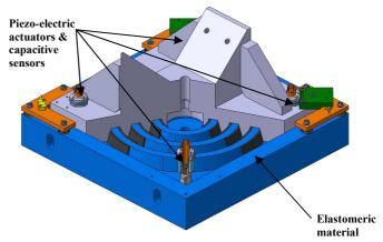
Figure 6. Scheme of the active feet
