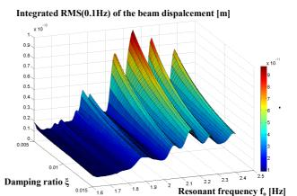
Figure 13. Integrated RMS(0.1Hz) versus mechanical support characteristics.
