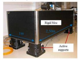
Figure 4. TMC table with STACIS feet
