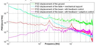
Figure 11. PSD obtained with feedback and adaptive control.
