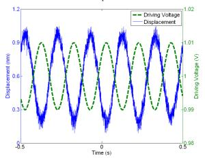
Figure 7. Voltage and displacement for the PPA10M actuator
