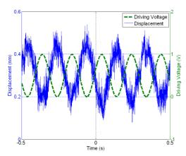
Figure 8. Voltage and displacement for the custom actuator
