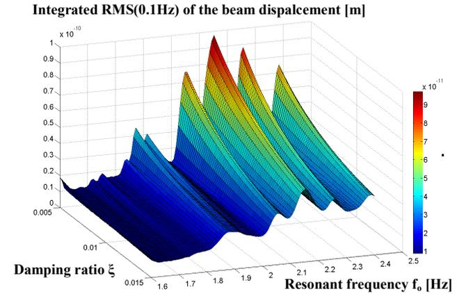
Figure 13. Integrated RMS(0.1Hz) versus mechanical support characteristics.
