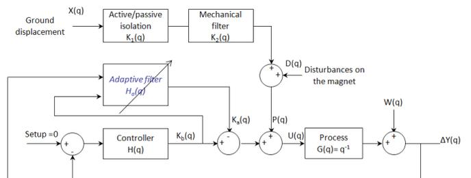
Figure 10. Scheme of the beam trajectory control.
