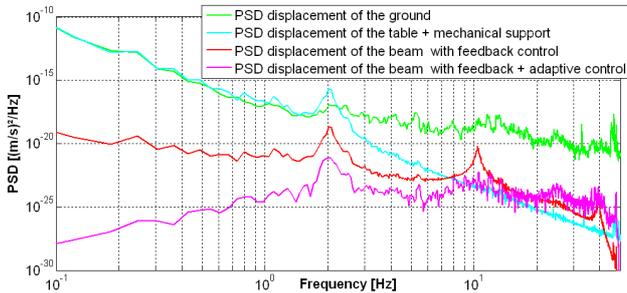
Figure 11. PSD obtained with feedback and adaptive control.
