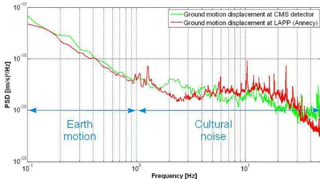
Figure 2. PSD displacement measured at LAPP and CMS site
