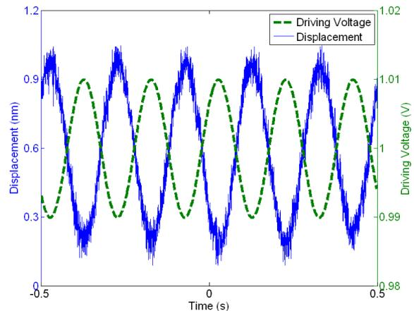
Figure 7. Voltage and displacement for the PPA10M actuator
