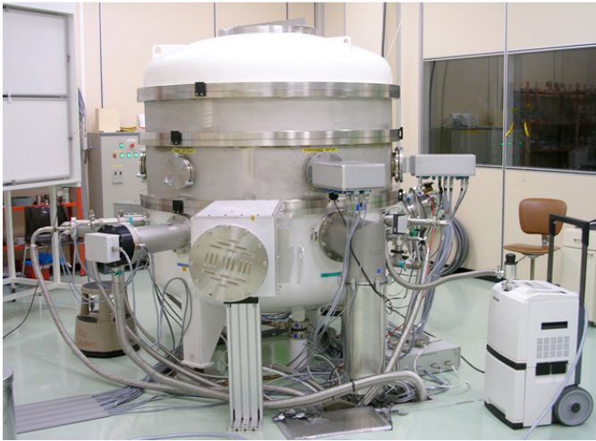
Fig. 6. The Saturne cryostat in the class 10 000 clean room. The two upper rings and the lid are removable for the integration of the calibration optics and the instrument. The optical port is on the opposite side.
