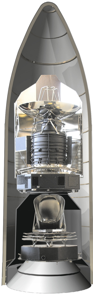
Fig. 10. An artist's impression of Herschel and Planck in launch configuration, under the fairing of the Ariane 5 rocket. Planck is attached to the rocket interface by means of a ring-shaped clampband. A cylindrical structure surrounds Planck and supports Herschel . Figure courtesy of ESA (C. Carreau).
