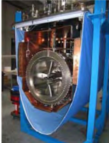
Fig. 8: The PLAVE SC-RFQ resonators in their cryostat.
