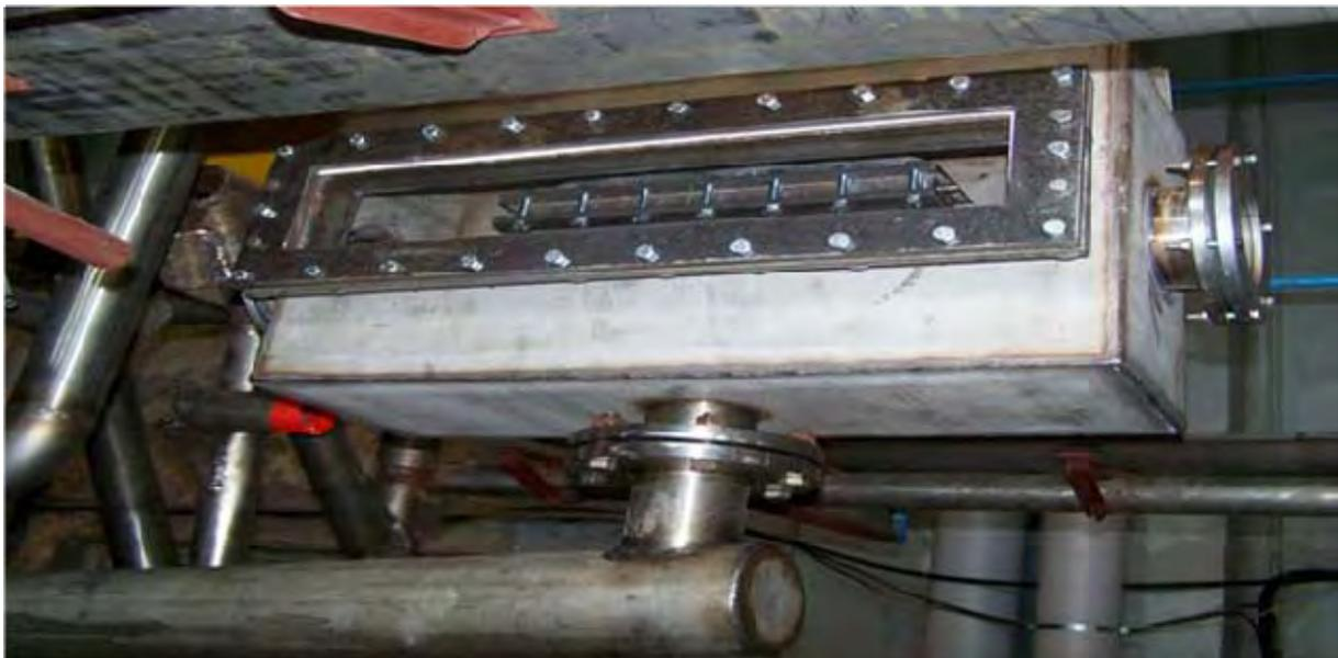
*Fig. 9: The VTF target on the test stand at IPUL, seen from below.*
