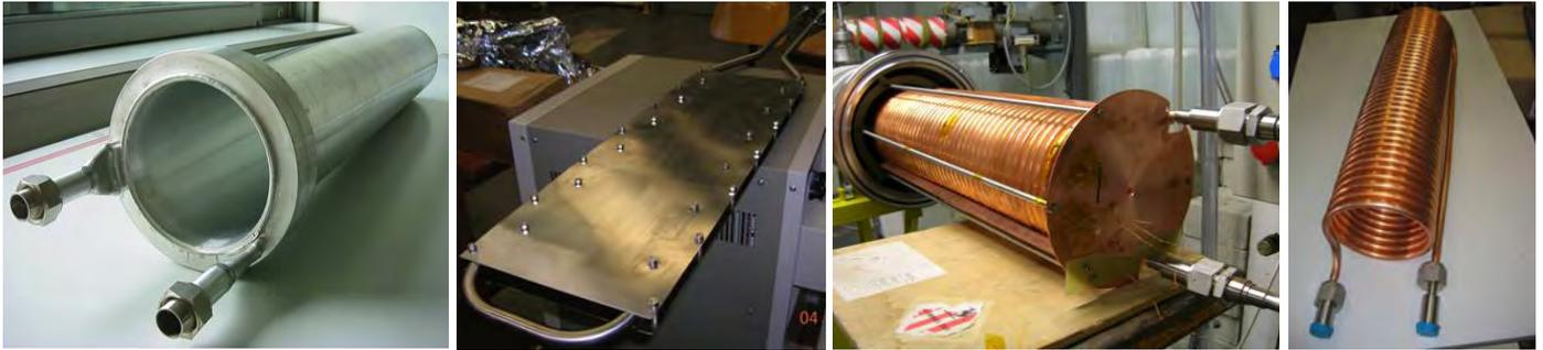
Fig. 8: Photographs of the various cryotrap prototypes.
