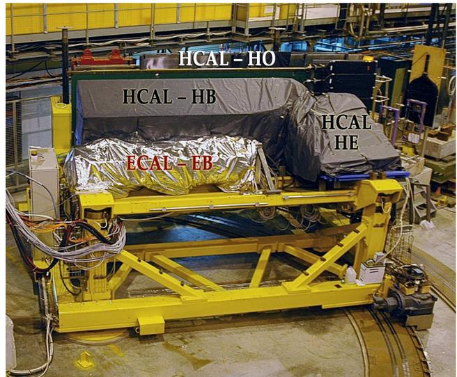
**Fig. 2.** The ECAL and the HCAL modules on a moving platform in the CERN H2 test beam area. The transporter table which supported the wedges is designed to move in  $\phi$  and  $\eta$  directions, approximately 0 to  $30^\circ$  in  $\phi$  and 0 to 3.0 in  $\eta$ .
