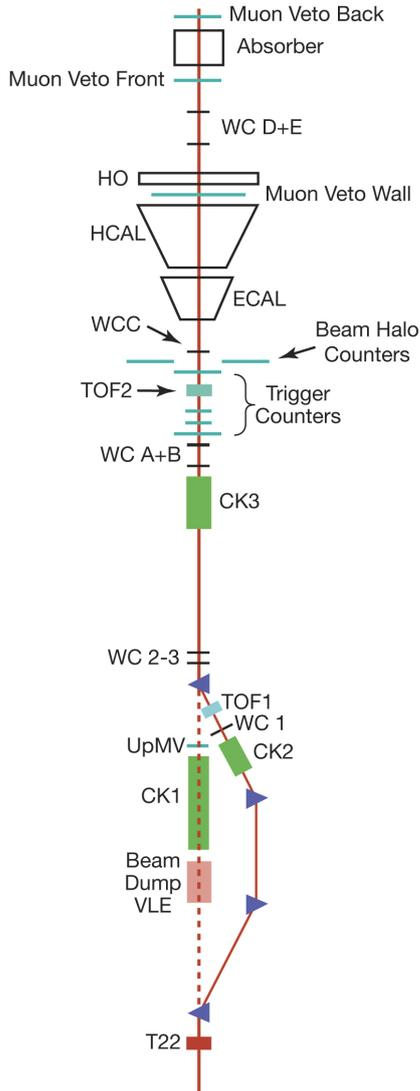
**Fig. 3.** The CERN H2 beam line and the experimental setup are shown schematically. In the VLE mode, the T22 target and a beam dump were inserted into the beam line, and the low energy particles were steered through the dog-leg.
