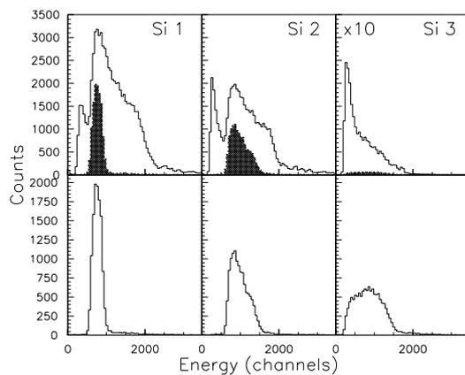
Figure 2: Raw energy spectra in the three silicon detectors: single spectra (solid lines in the top row) and coincident spectra (bottom row and hatched areas in the top row). The number of counts in the upper right histogram has been divided by a factor 10.
