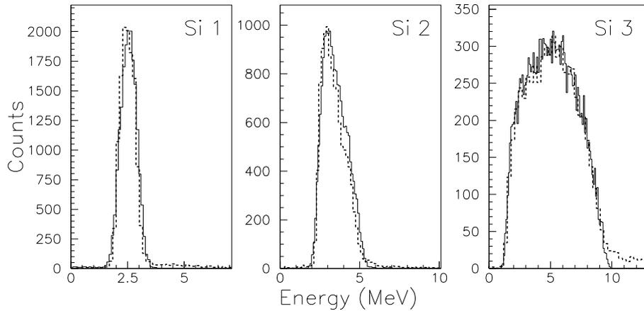
Figure 3: Measured (dashed lines) and simulated (solid lines) energy spectra of recoil protons in the silicon detectors.
