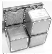
(b) Front-view of the prototype EC, with three of the MAPMT installed.
