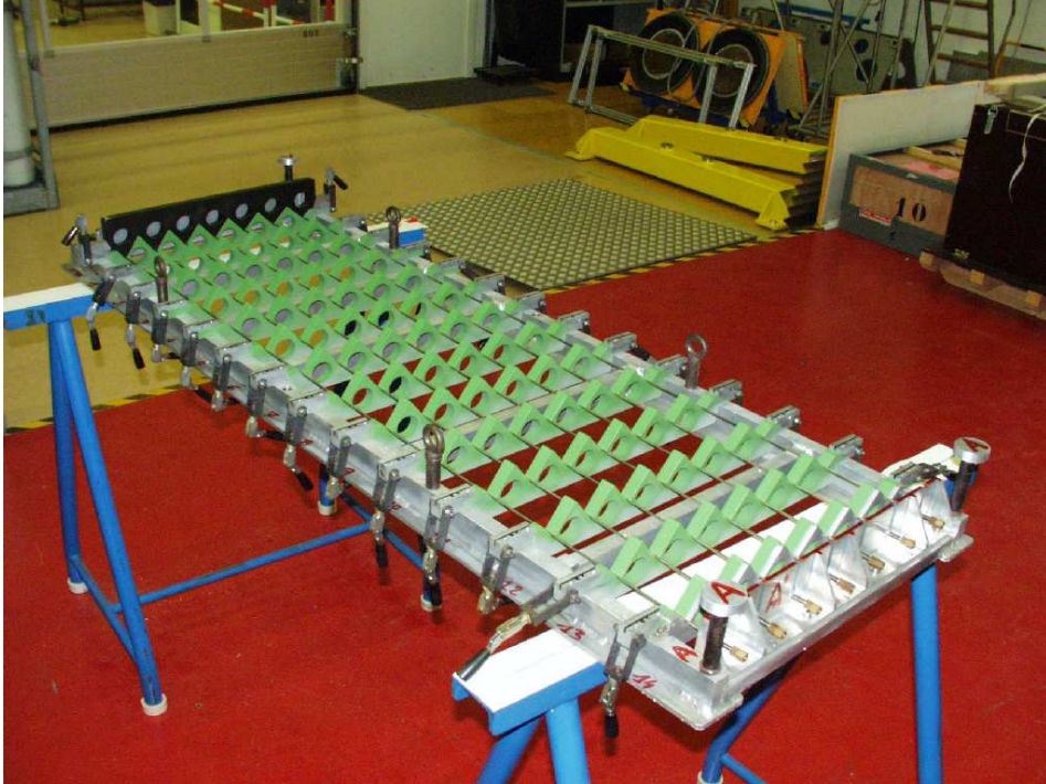
Fig. 16. Tooling used to produce a spacer.
