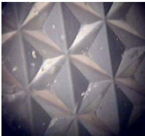
Fig. 13. Photographs of the micro prisms retro reflective target
