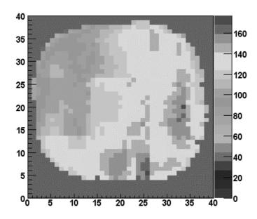
Figure 2 represents the 41 x 41 map of FEP values: the FEP channel varied from 80 to 170 keV from one pixel to another.
