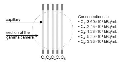
Figure 3. Geometry and characteristics of the capillary phantom.
