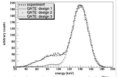
Figure 8 shows the experimental energy spectrum for the <sup>99m</sup>Tc point source and the different energy spectra obtained by simulating different designs of the scintillation camera.
