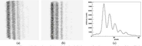
**Figure 10.** Experimental (a) and simulated (b) images of a phantom consisting of 5 capillaries filled with <sup>99m</sup>Tc solutions of different concentrations and horizontal profiles through these images (c: experimental in dashed line and simulated in solid line).
