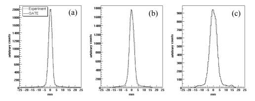
**Figure 4.** Measured and GATE simulated point spread functions for a centred  $^{99m}$ Tc point source located at (a) 2cm ,(b) 5 cm and (c) 10 cm from the camera.
