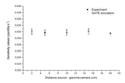
**Figure 7**. Comparison between experimental and simulated system sensitivity for the centred <sup>99m</sup>Tc point source, for 5 distances between the source and the scintillation camera collimator.
