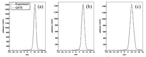
**Figure 5.** Measured and GATE simulated point spread functions for a  $^{99m}$ Tc point source 1 cm off-axis and located at (a) 2cm ,(b) 5 cm and (c) 10 cm from the camera.
