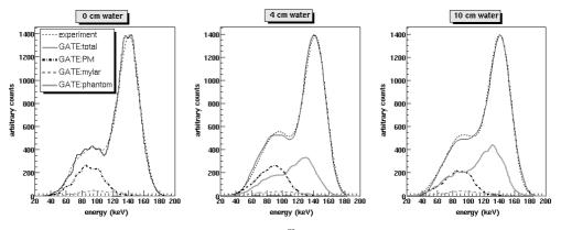
Figure 9. Energy spectra obtained for the <sup>99m</sup>Tc point source at 12 cm from the collimator under a water thickness of 0, 4 and 10 cm.
