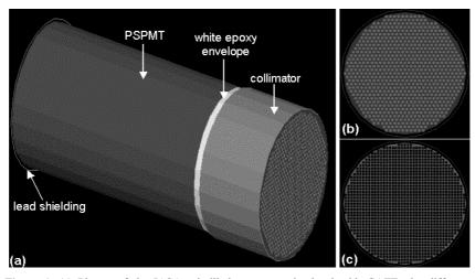
**Figure 1.** (a) Picture of the IASA scintillation camera simulated with GATE: the different components of the detector head are represented (collimator, white epoxy envelope surrounding the crystal, PSPMT and shielding); (b) the hexagonal hole collimator geometry; (c) the CsI(TI) crystal array geometry.
