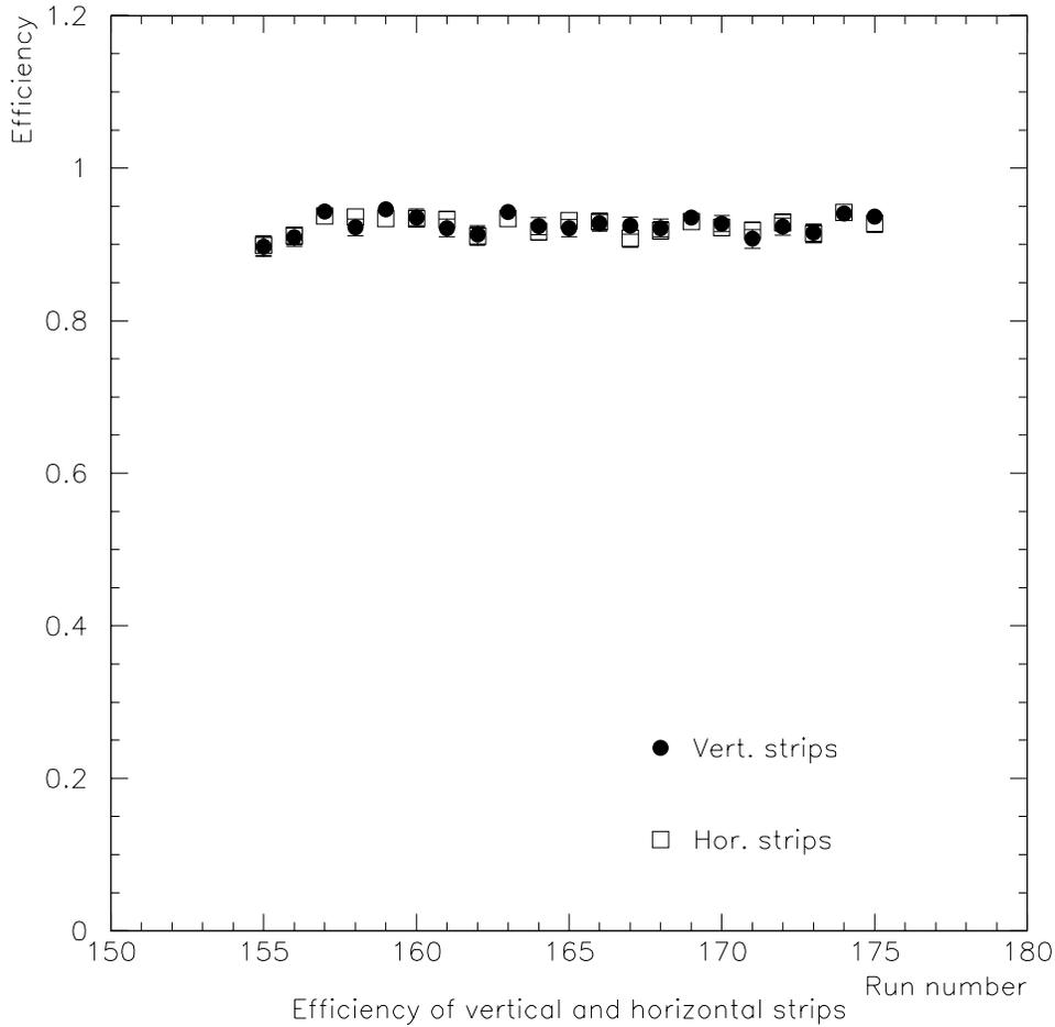
Fig. 4. Cosmic rays efficiency measured at the GIF for a uniform counting rate of about  $300 \text{ Hz/cm}^2$  at 9.4 kV
