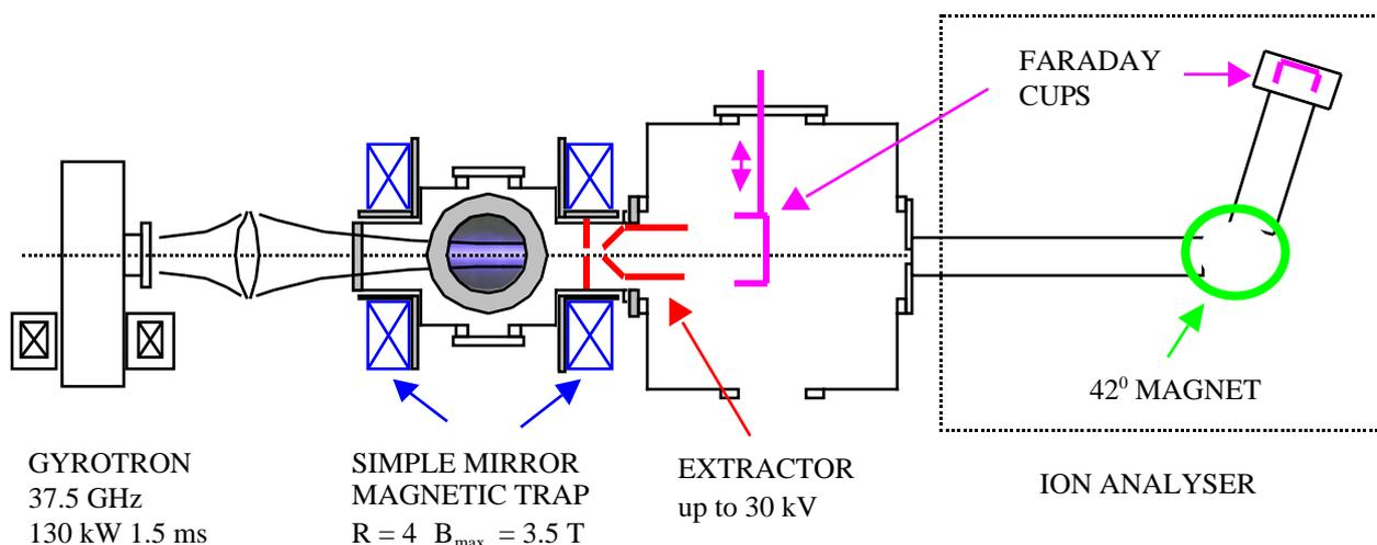
Figure 1: Schematic presentation of the setup SMIS 37
