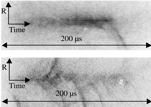
Figure 7: Negative streak camera images. Upper one is for the discharge with 200 mA/cm<sup>2</sup> of extracted current, lower - with 2 A/cm<sup>2</sup>.
