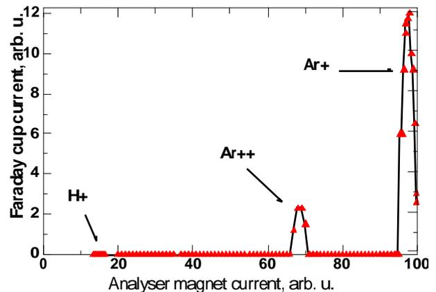
Figure 9: Ion charge state distribution in off-resonant discharge.
