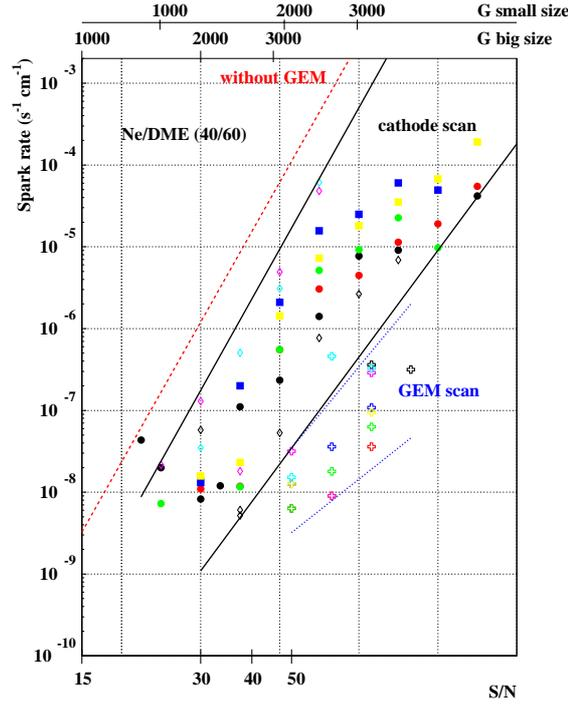
Fig. 3. Spark rate as a function of the signal to noise ratio and corresponding gain. Cathode scan (dashed line) of the chambers without GEM [3]. Cathode scan with  $\Delta V_{GEM} = -360V$ . GEM scan with  $V_K = -360V$  (cross symbols). (At  $S/N = 30$ :  $V_K = -360V$ ,  $\Delta V_{GEM} = -360V$ )
