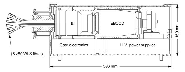
Figure 7: Optoelectronic chain used to read six detector modules. The chain comprises an image intensifier (II) and an electron-bombarded CCD (EBCCD).
