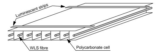
Figure 1: Schematic view of the polycarbonate cells and WLS fibres in a section of a detector module. Each cell has a cross-section of  $0.9 \times 1.1$  cm<sup>2</sup> and a length of 6 m. The electro-luminescent strips are used for calibration.
