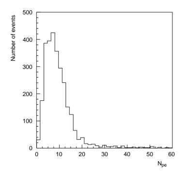
Figure 9: Distribution of number of photoelectrons,  $N_{pe}$ , emitted at first photocathode of EBCCD chain for minimum-ionizing particles crossing a module at a distance d = 4.3 m from the fibre readout ends.
