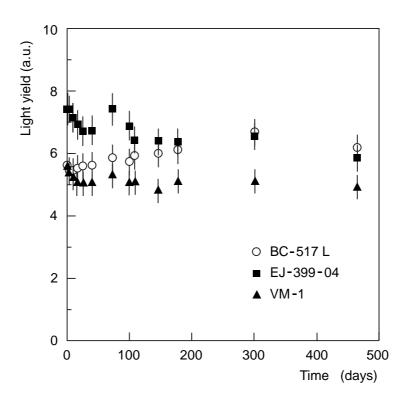
Figure 6: Long-term stability of a WLS fibre immersed in three liquid scintillators, and irradiated at room temperature using a  $^{90}$ Sr source.
