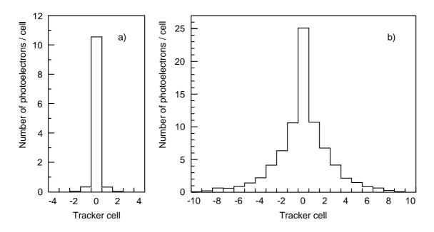
Figure 13: Intensity profiles, averaged over many events, for incoming  $e^-$  of 4 GeV: a) with no lead present; b) with 5.6 cm of lead in front of tracker.
