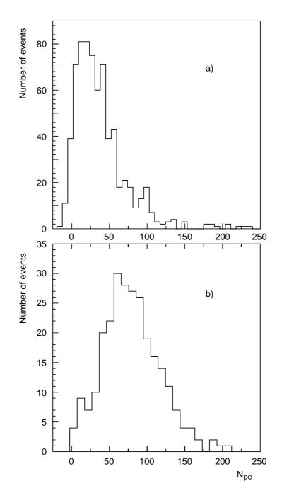
Figure 12: Distributions of numbers of photoelectrons,  $N_{pe}$ , emitted at first photocathode of EBCCD chain, for showers generated in 5.6 cm of lead by: a) 2 GeV  $e^-$  and b) 4 GeV  $e^-$ . The line of flight of the incoming electrons crosses the module at a distance d = 4.3 m from the fibre readout ends. For each fired cell the average background per cell has been subtracted, resulting in negative values of  $N_{pe}$  in a small fraction of cases.
