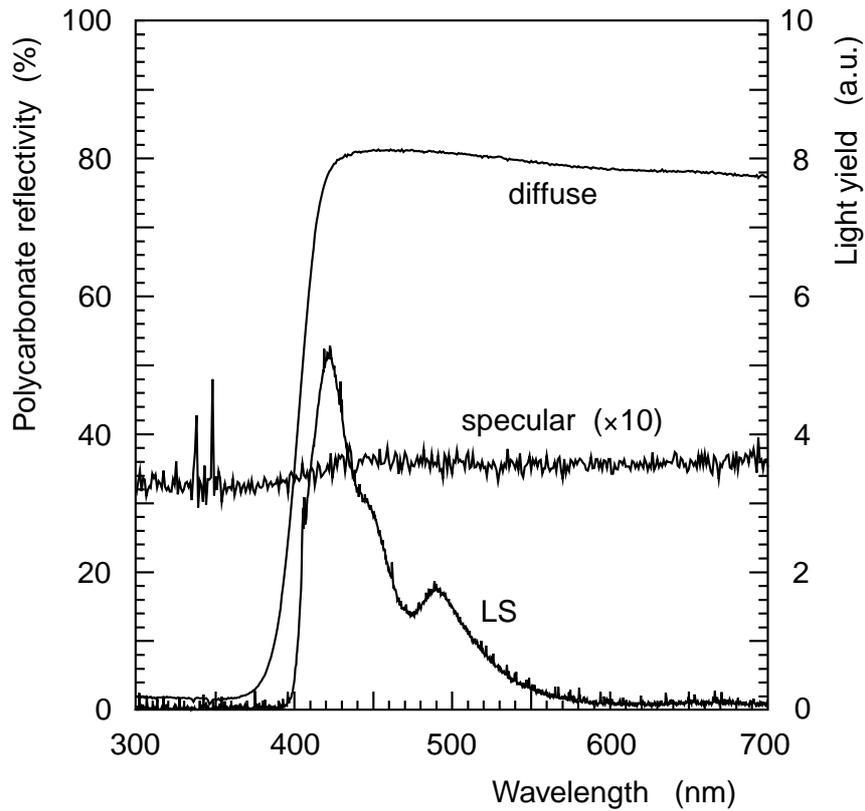
Figure 2: Reflectivity as a function of wavelength for polycarbonate doped with 20 %  $\text{TiO}_2$ , with specular and diffuse components shown separately (left scale). The emission spectrum for the liquid scintillator (LS) BC-517L doped with 0.7 % naphthalene is superimposed (right scale).
