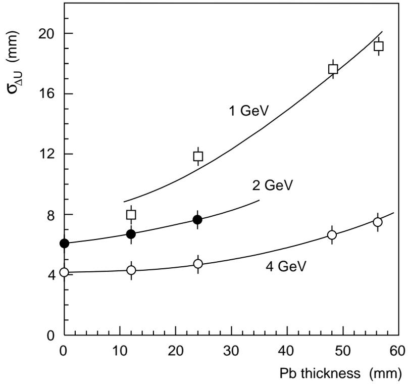
Figure 15: Variation with lead thickness and  $e^-$  energy of the standard deviation,  $\sigma_{\Delta U}$ , characterising the distribution of the difference between particle position given by wire chambers and shower position given by LS tracker module. Curves are drawn to guide the eye.
