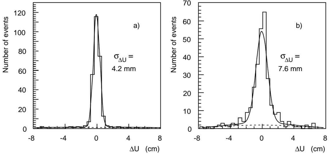
Figure 14: Distribution of difference,  $\Delta U$ , between particle position given by wire chambers and shower position given by LS tracker module, for incoming  $e^-$  of 4 GeV: a) with no lead present; b) with 5.6 cm of lead in front of tracker. Each distribution is fitted by a Gaussian, of standard deviation  $\sigma_{\Delta U}$ , superimposed on a broad background.
