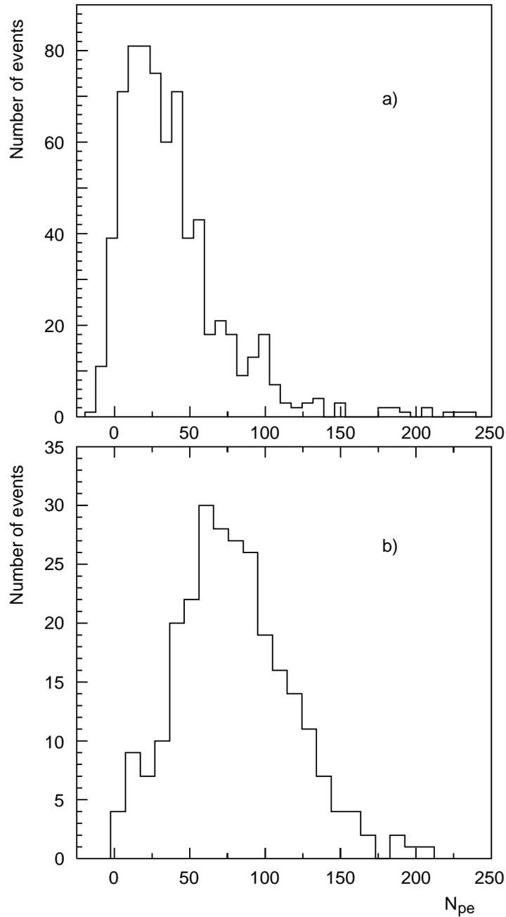
Figure 12: Distributions of numbers of photoelectrons,  $N_{pe}$ , emitted at first photocathode of EBCCD chain, for showers generated in 5.6 cm of lead by: a) 2 GeV  $e^-$  and b) 4 GeV  $e^-$ . The line of flight of the incoming electrons crosses the module at a distance  $d = 4.3$  m from the fibre readout ends. For each fired cell the average background per cell has been subtracted, resulting in negative values of  $N_{pe}$  in a small fraction of cases.
