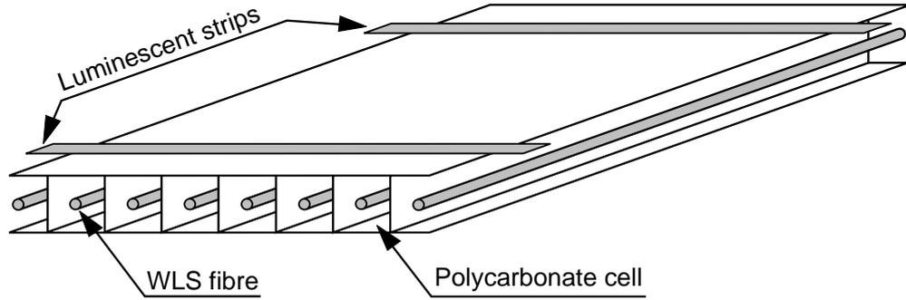
Figure 1: Schematic view of the polycarbonate cells and WLS fibres in a section of a detector module. Each cell has a cross-section of  $0.9 \times 1.1 \text{ cm}^2$  and a length of 6 m. The electro-luminescent strips are used for calibration.
