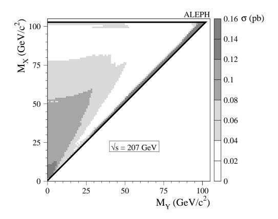
Figure 9: The 95% C.L. upper limit on the production cross section in pb for the process  $e^+e^- \to XX \to YY\gamma\gamma$  multiplied by the square of the branching ratio  $\mathcal{B}(X \to Y\gamma)$ .
