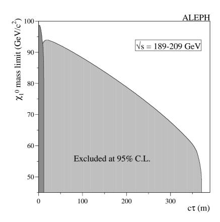
Figure 5: The excluded regions in the plane of the  $\chi_1^0$  mass versus  $\chi_1^0$  proper lifetime, at 95% C.L., for the reaction  $e^+e^- \to \chi_1^0 \chi_1^0 \to \tilde{G} \tilde{G} \gamma \gamma$ , under the assumptions of the MGM. The lighter shaded region is based on the search for single photons which do not originate from the interaction region (Section 4.6); the darker shaded region is based on the search for acoplanar photon pairs (Section 5.2).
