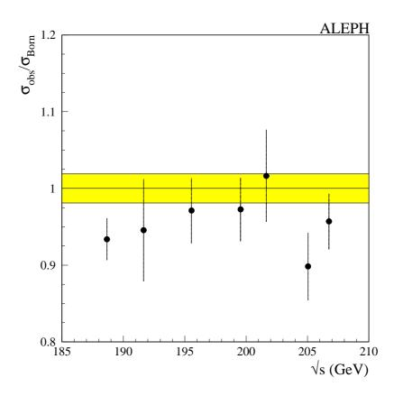
Figure 11: The ratio of observed to Born cross section as a function of centre-of-mass energy for the process  $e^+e^- \to \gamma\gamma$ , for the acceptance region  $|\cos\theta^*| < 0.95$ . The shaded region represents the common systematic uncertainty of  $\pm$  1.9%.
