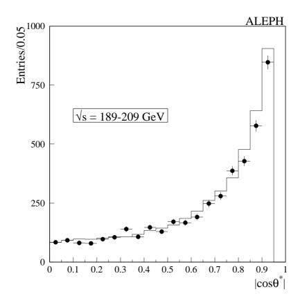
Figure 10: Predicted (histogram) and observed (points with error bars ) angular distributions for the reaction  $e^+e^- \to \gamma\gamma$  as a function of  $|\cos\theta^*|$ , where  $\theta^*$  is the photon production angle in the two-photon rest frame. The errors shown here are purely statistical.
