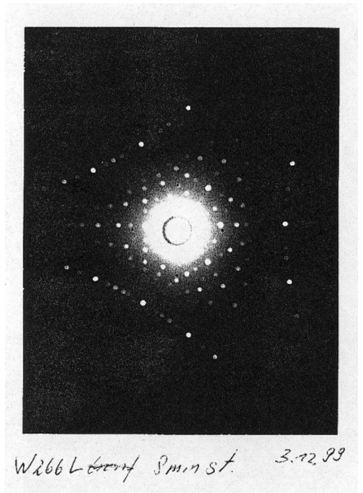
8 mm crystal Laue diffraction pattern
