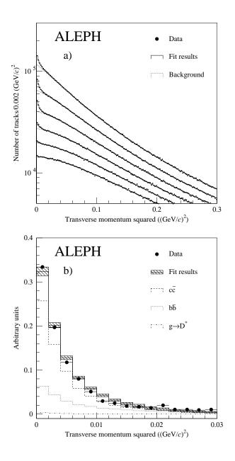
Figure 1: a) Transverse momentum squared of tracks in 0.5 GeV/c momentum bins from 1 GeV/c (uppermost) to 4 GeV/c. The signal peaks in the low- $p_{\rm T}^2$  region. b) Signal  $p_{\rm T}^2$  distributions, determined as described in the text, are shown. The hatched rectangles represent the Monte Carlo prediction within errors. In the error the uncertainty concerning the offset on the rate is not included.
