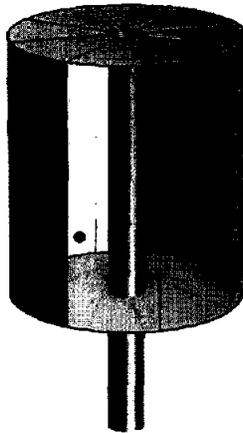
Figure 2: Eight-fold segmented true-coaxial Ge detector with four simulated interactions of  $\gamma$ -radiation with the detector shown as full circles.
