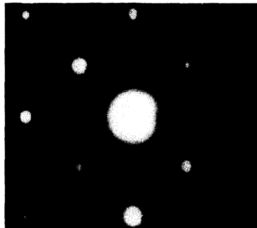
FIG. 4. Electron diffraction pattern of a LPCVD Si layer on sapphire after laser annealing with a 30-ns pulse from the Q -switched Nd : YAG laser at a fluence of 3 \text{ J cm}^{-2} and after removing the sapphire substrate.
