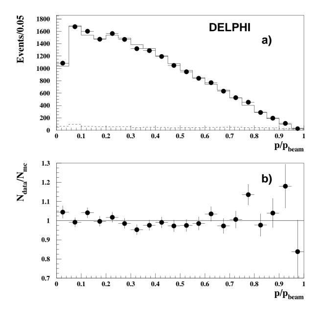
Figure 13: a) momentum distribution for identified electrons. The points are data, the full line is the expectation from simulation, and the dashed line is the simulated background contribution. b) The ratio between data and the expectation from simulation.
