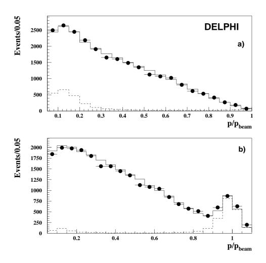
Figure 7: Momentum distribution of the sample of  $\mu$  candidates when all the requirements of the analysis are applied except: a) the isolation angle criterion and b) the  $p_{rad}$  requirement. The full line shows the expectation from simulation. The dashed line shows the expected background contamination.
