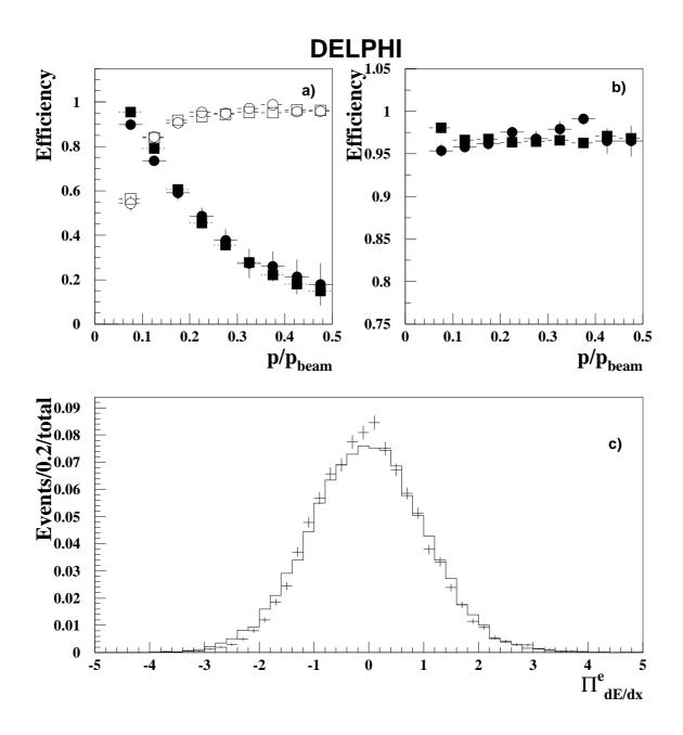
Figure 14: Example of efficiency checks, for the electron sample from 1994. a) Efficiency of the  $\Pi_{E/p}$  (open marks) and  $\Pi_{dE/dx}^{\pi}$  (solid marks) requirements as a function of momentum. b) The efficiency estimated from the logical sum (the '.OR.') of these requirements. The circles represent simulation, the squares are for data. c)  $\Pi_{dE/dx}^{e}$  for a selected sample of Bhabhas. The crosses represent the data, the full line histogram corresponds to the simulation.
