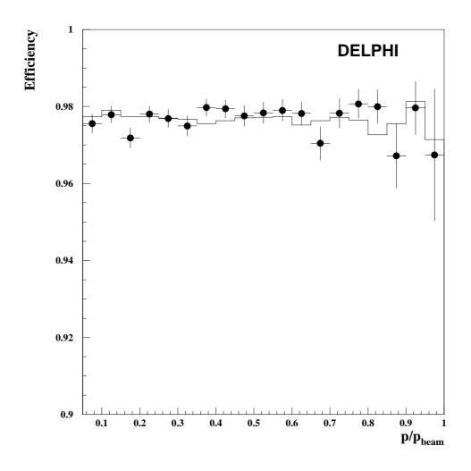
Figure 6: Comparison of data (points) and simulation (full line) for the estimate of the identification efficiency of the combined HCAL and muon chamber requirement.
