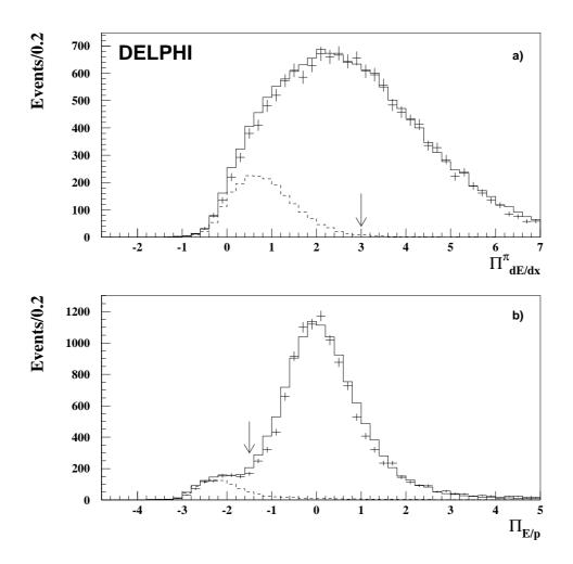
Figure 11: Distributions of variables used for electron identification in the momentum range  $0.05 < p/p_{beam} < 0.5$ : a)  $\Pi_{dE/dx}^{\pi}$ , b)  $\Pi_{E/P}$ . Events are accepted for further analysis if at least one of the variables has a value above those indicated by the arrows. The points represent the data, the full line results from the simulated sample and the dashed line shows the background contribution.
