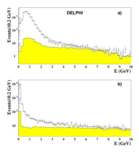
Figure 9: Distributions of a) the average energy deposition per layer in the HCAL, and b) the total electromagnetic energy in a cone with half opening angle of 18° around the muon candidate track. The crosses show the data, while the full line shows the simulation result. The shaded area shows the contribution from backgrounds.
