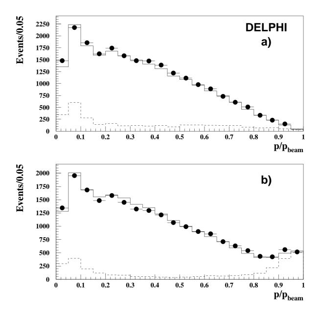
Figure 15: Momentum distribution for identified electrons with a) no isolation angle requirement and b) no  $E_{rad}$  requirement. The points are data, the full line is the expectation from simulation and the dashed line is the simulated background contribution.
