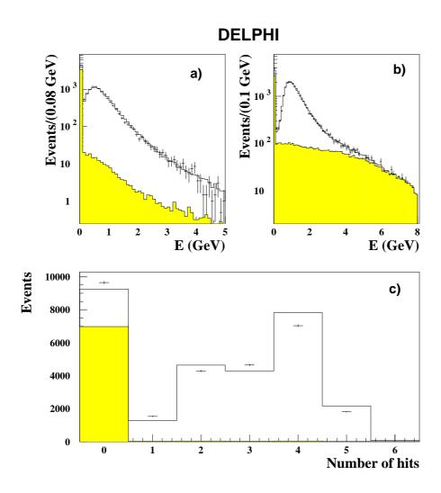
Figure 5: Muon identification variables: a) The energy of the outermost HCAL layer, b) largest HCAL energy deposition and c) the number of associated hits in the muon chambers. The crosses represent the data, the full line histograms represent the simulated events and the shaded areas are the non- $\mu$  contributions. All requirements described in the text were applied, except the one corresponding to the distributed variable.
