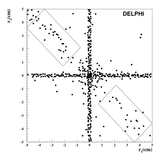
Figure 4: The impact parameter of the leading track in one hemisphere plotted against the impact parameter of the leading track in the other hemisphere. The number of events found inside the rectangles is used to estimate the number of cosmic ray events in the selected sample.
