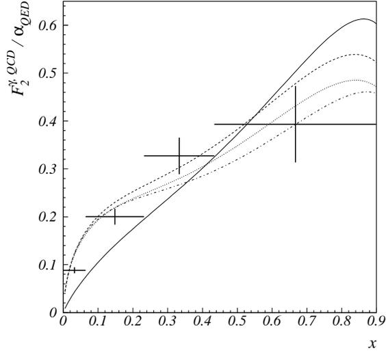
**Fig.3** Test of the unfolding of  $F_2^{\gamma,FKP}$  made at the generator level. The crosses are the unfolded result. The curves are the unfolded result. The solid curve shows the  $F_2^{\gamma,QPM}$  dependence while other curves show  $F_2^{\gamma,FKP}$ , the input distribution calculated under different assumptions for the mass of the target photon, as discussed in the text.
