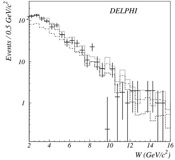
**Fig.6** Comparison of the invariant mass distributions for the data drawn by the crosses and the simulation. The histograms show the predictions for GS [21] (dashed), DO [22] (dotted) and LAC1 [20] (dashed-dotted) parameterizations.
