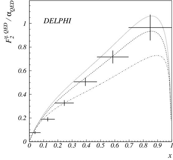
**Fig.4** Unfolded  $F_2^{\gamma,QED}$ . The crosses are the unfolded result. The curves show  $F_2^{\gamma,QED}$  calculated under different assumptions for the mass of the target photon: upper curve with zero mass, middle curve, using values from simulated data, lower curve taking the average value.
