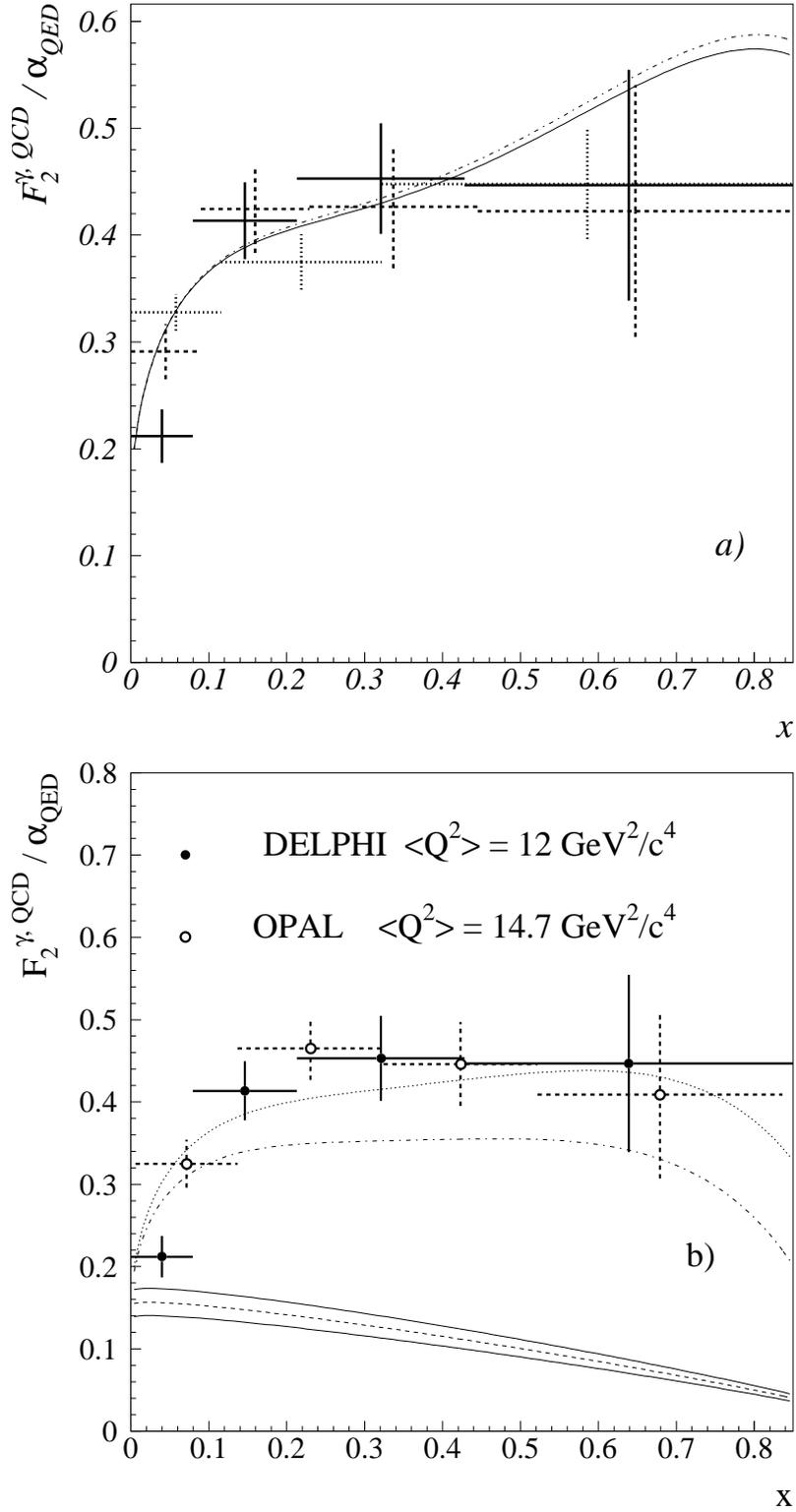
**Fig.7** (a) Unfolded  $F_2^\gamma$  from light quarks simulated data for the different approaches drawn by the crosses and described in the text. The solid (dashed-dotted) curve presents the sum of the GVDM and FKP' prediction for the QCD scale parameter  $\Lambda$  equal to 0.3 GeV (0.2 GeV).
